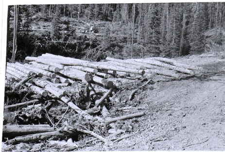
Picture No. 9, taken in the same locality as the one above, shows a deck of transmission poles that had been sorted out of the tree-length stems skidded to the slashersaw-loader at the landing. In this area, in addition to pulpwood and transmission poles, the contractor also was hauling the larger 100-inch bolts to a stud mill in White Sulphur Springs. However, such diversification in lodgepole pine logging is not common and in this case was occasioned by cutbacks in pulpwood orders.
