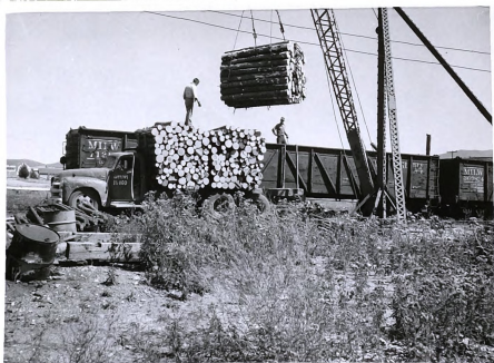
Picture 46 shows the transfer of pulpwood from truck to gondola car at the railhead at White Sulphur Springs, Montana. The pulpwood on the truck is divided in three sections by removable stakes. This helps in loading, tends to prevent side slippage enroute, and provides space to slip the sling over the ends as shown in unloading. Less than ten minutes is required to unload a truck by this method.
