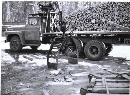
Pictures 37 and 38 show two clamshell-type pulpwood loaders. Robert Larson, Diesel Power Equipment, Ely, Minnesota, distributor for the Hyabob Hydraulic Loader, supplied the upper picture of the machine in operation. The lower picture shows the experimental machine made by Charles Erickson and Son for their Idaho Pulpwood operation.
