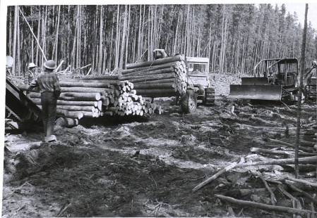
Pictures 18-20 show prehauling of bundles of 100-inch pulpwood from stacked ricks on the Heggie Bros. operation north of Martinsdale, Montana. The upper picture shows how the wood is stacked by the fallers over a bolt placed at one end to provide cable passage. The lower pictures show how the ricks are winched upon an arch for delivery to the loader. This method of logging was not timed in this study.
