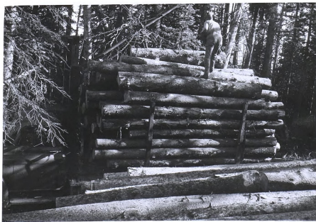
Pictures 39 and 40 are before-and-after loading views of a self-loading truck for hauling sawlogs. The upper picture shows the winch mechanism. Pulling on the long, rope-control powers the winch and lifts the logs over the side. Tongs are placed in the middle of the log as shown in the lower picture. The loading device was made and installed by Wilson Lowry, trucker for the Otto Lumber Co., Laramie, Wyoming.
