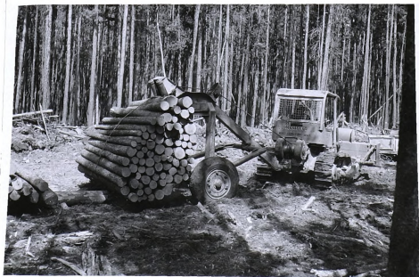
Pictures 18-20 show prehauling of bundles of 100-inch pulpwood from stacked ricks on the Heggie Bros. operation north of Martinsdale, Montana. The upper picture shows how the wood is stacked by the fallers over a bolt placed at one end to provide cable passage. The lower pictures show how the ricks are winched upon an arch for delivery to the loader. This method of logging was not timed in this study.
