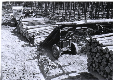
Pictures 27 and 28 show two views of the side-to-side, chain-lift loader used by Heggie Bros. north of Martinsdale, Montana. The upper member of the machine can be raised or lowered by an hydraulically activated piston (visible underneath) so the logs do not drop so far onto the truck. The gasoline engine that powers the chain is situated between the wheels and the inclined ramp. Two men feed logs to the loader and the trucker stacks his own load as shown. The pulpwood is delivered to the loader by tractor and arch as shown in the lower picture and in pictures numbered 18-20.
