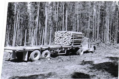
Picture 47 shows a flatbed trailer modified for lengthwise hauling of pulpwood by Heggie Bros., White Sulphur Springs, Montana.
