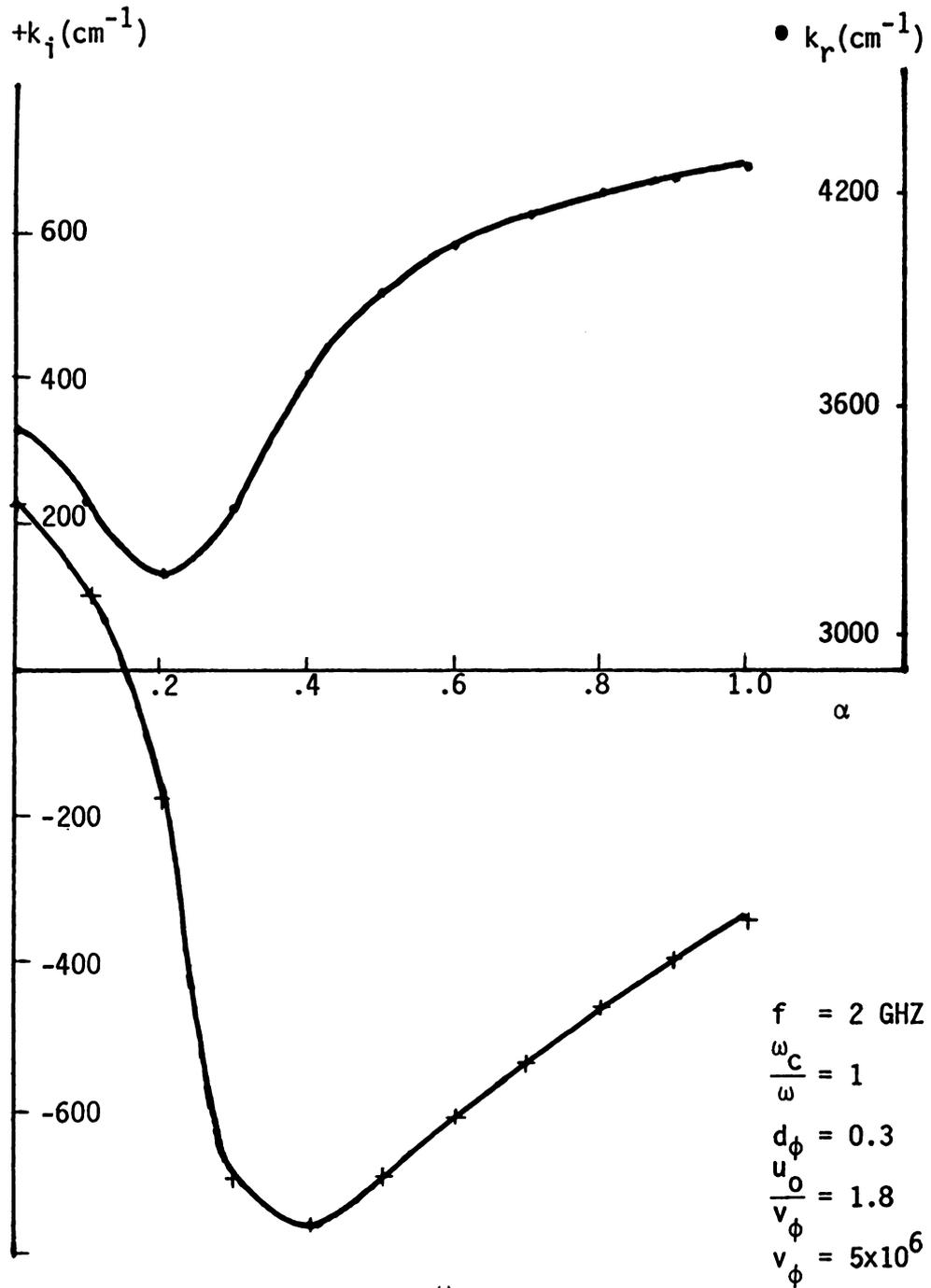
Figure 12.  $k$  vs.  $\alpha$  ( $\frac{\omega_c}{\omega} = 1$ ) of case II
