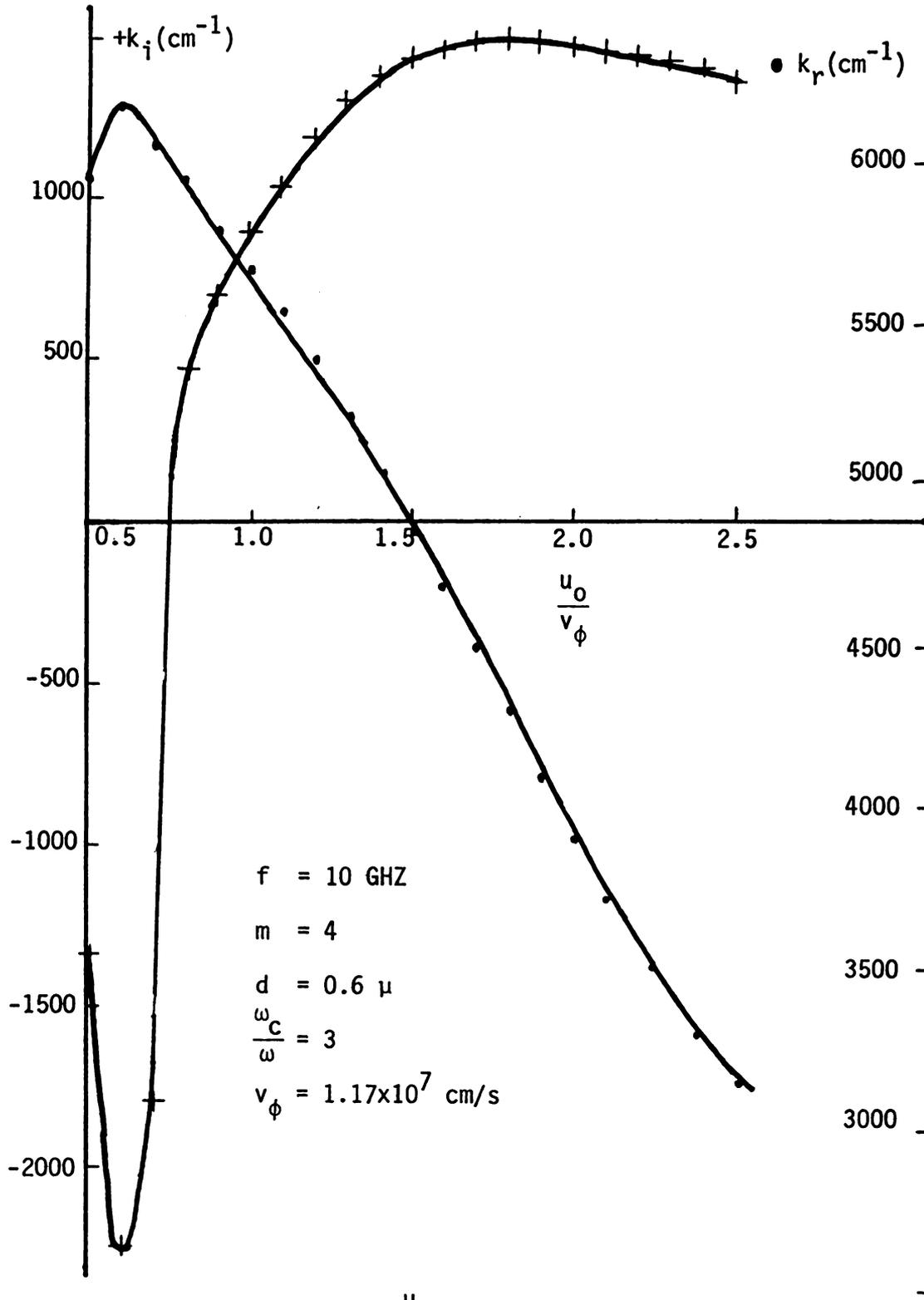
Figure 22.  $k$  vs.  $\frac{u_0}{v_\phi}$  in the ripple boundary case
