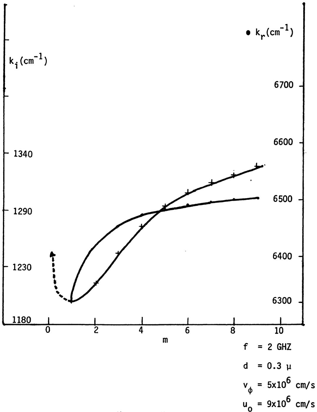
Figure 20.  $k_i$  vs.  $m$  ( $\frac{\omega_c}{\omega} = 1$ ),  $\frac{\omega_c}{\omega} = 1$  (ripple boundary case)
