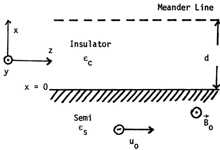
Figure 1. Semi-infinite semiconductor and meander line
