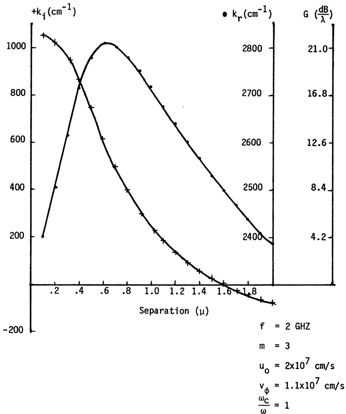
Figure 21.  $k$  vs. separation in the ripple boundary case
