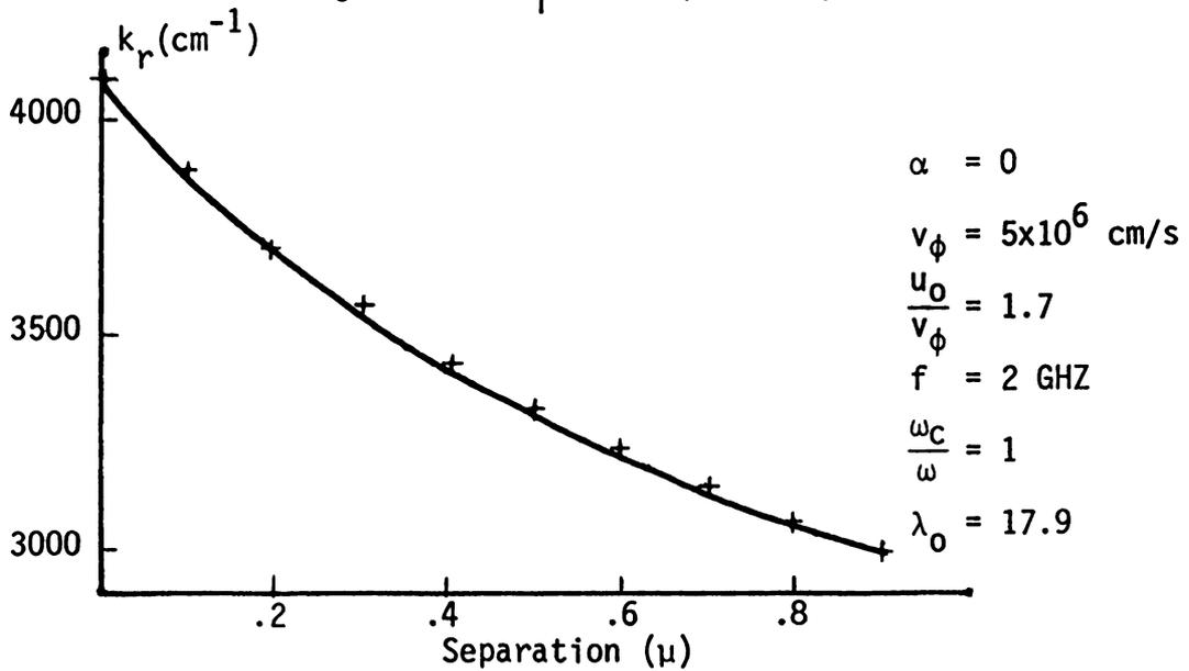
Figure 15. Wavenumber at maximum gain vs.  $d$  (case II)
