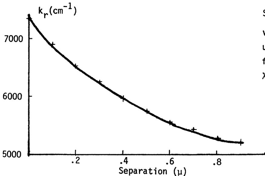
Figure 9. Wavenumber at maximum gain vs.  $d$
