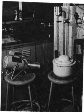
Figure 19. Special equipment used to control the relative humidity in the 75 degree Fahrenheit room.
