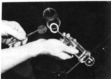
Figure 17. Positioning device for exposing leaf sample to mist.
