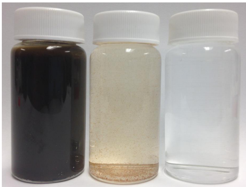
Figure 3.7. Color change of the solution following different treatment stages Left to right: AD effluent, EC effluent and membrane filtrate.
