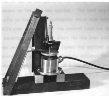
Figure 8. Device for conducting relaxation experiments of alfalfa stem sections
