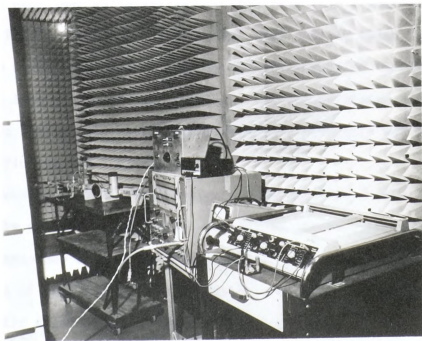
Figure 5.31 Photograph of Surface-Field Measurement System.
