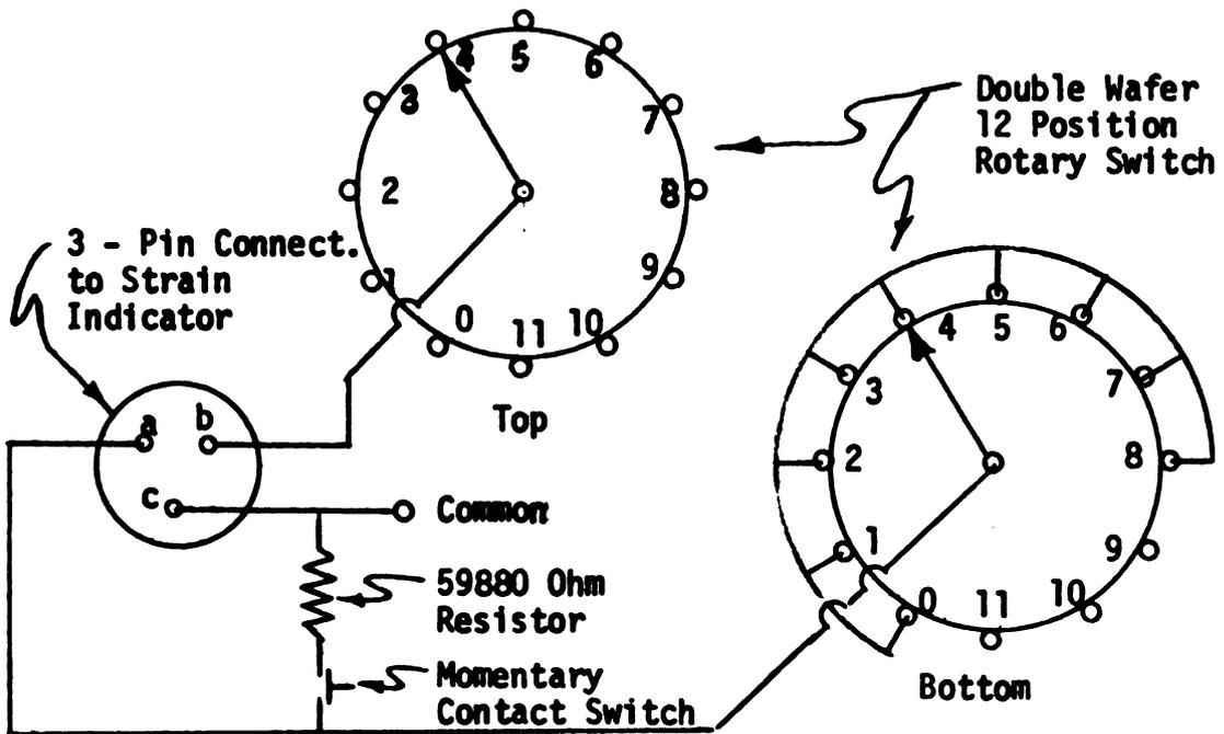
Figure 12 - Switching Unit Wiring Diagram - 1972
