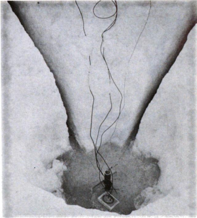
Figure 5 - Attachment of Strain Gages to Poles
