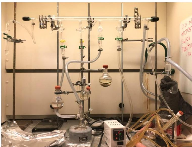
Figure 2.3: Schlenk line setup for functionalization of Si NCs.
