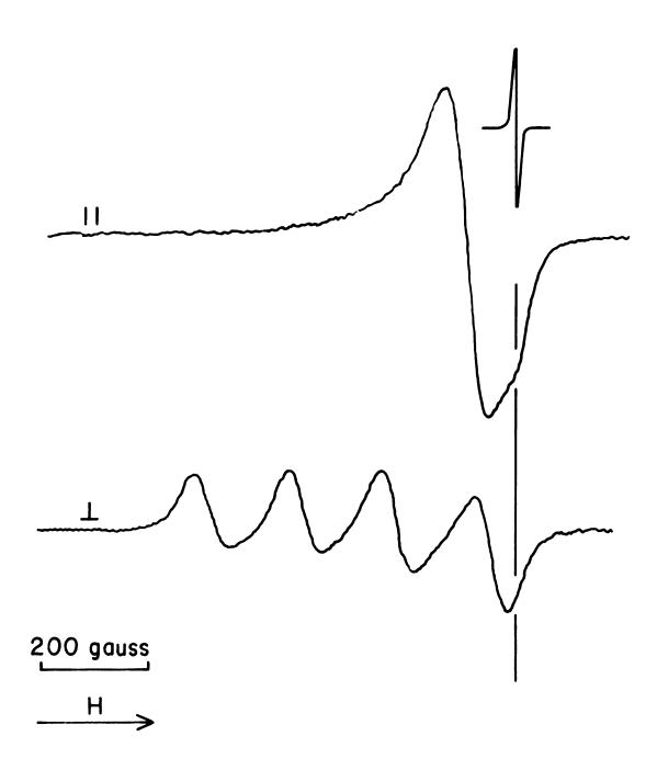
smectite. In Cu(bp)<sub>2</sub><sup>2+</sup> and the Cu(bp)<sub>3</sub><sup>2+</sup> cation at 100°C, where the complex is in contact with the clay surface, spin-lattice relaxation mechanisms may cause broadening of the nitrogen hyperfine lines so they do not appear. In the tris complex at 77 percent r.h. the broadening is probably due to rapid molecular tumbling.
