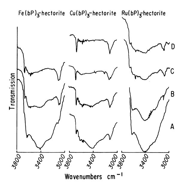
Figure 6.--Infrared spectra of Fe(bp) $_3^{2+}$ , Cu(bp) $_3^{2+}$  and Ru(bp) $_3^{2+}$  hectorite (two symmetry additions) from 3800 cm $^{-1}$  to 3000 cm $^{-1}$ at (A) 30% r.h., (B) 100°C and (C) 200°C.
