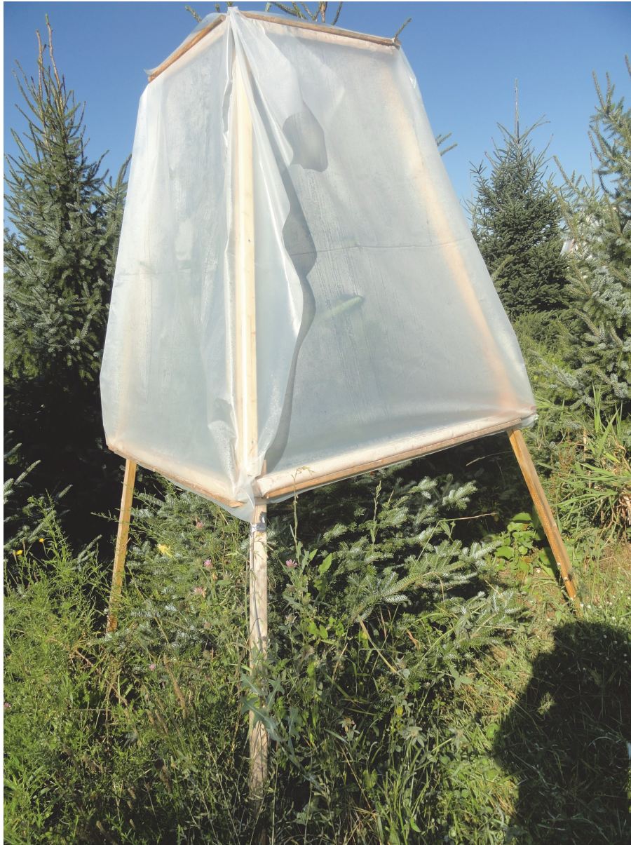
Figure 5.2. Polyethylene tent used for solar heating of upper tree canopy.
