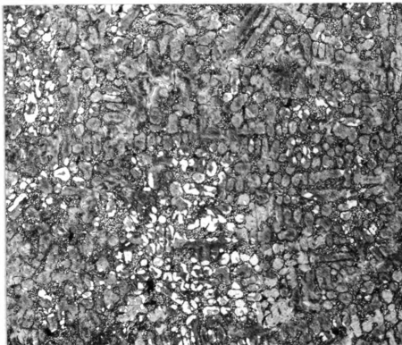
Fig 16. Microstructure of Iron T13-M, Treated with Magnesium. Nital 100x.
