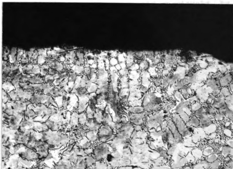
Fig 11. Structure at the Surface of Iron T2-F2, Treated with .6% Ferro-silicon. Nital 100x.
