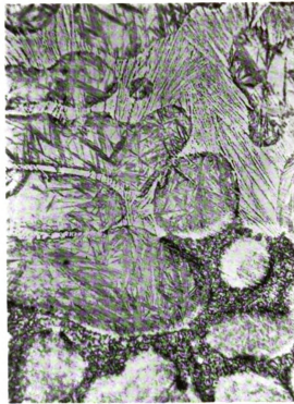
Fig. 1—Acicular carbide and undercooled graphite. Etched in picral 300
