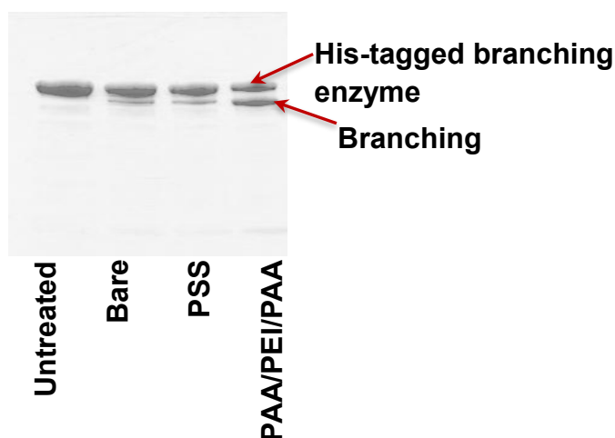
Figure 3.9. SDS-PAGE analysis of His-tagged SUMO branching enzyme proteolysis during passage through bare, PSS-, PAA/PEI/PAA-modified nylon membranes that contained His-tagged SUMO protease. The residence time in the membrane was \sim 0.17 s.
