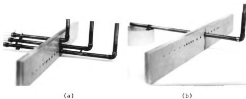
FIGURE 15 (a) One-Half Inch Capture Tube (b) Three-Eighths Inch Capture Tube
