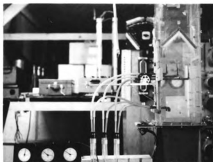
FIGURE 14 Droplet Capture Tube Apparatus
