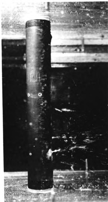
FIGURE 41 Boundary-Layer Separation for Gas Reynolds Number equal 5.6 \times 10^4 and Water Pressure equal 20 psig at Spray Nozzle
