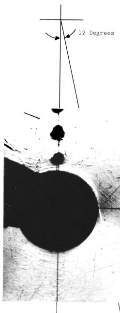
FIGURE 17 Boundary-Layer Separation in Single-Phase Flow with Forward Stagnation Point at Top of Cylinder, Reynolds Number equal 5.64 \times 10^4
