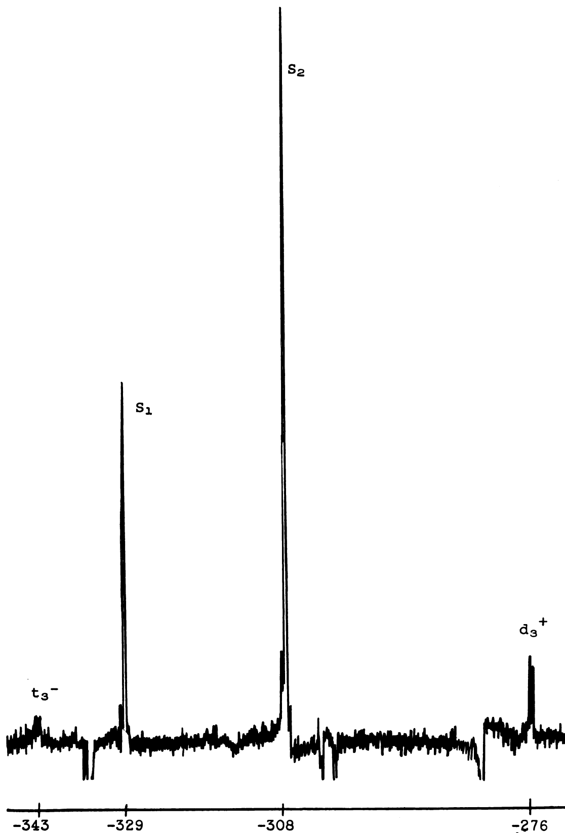
Figure 12. ^{19}\text{F} magnetic resonance of 0.36\text{ M TiF}_4 + 0.72\text{ M TiCl}_4/\text{THF} at -60^\circ\text{C} . (Internal reference: TFA)
