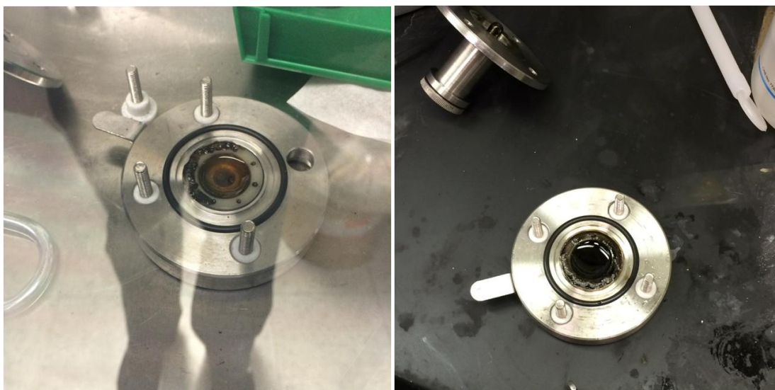
Figure 4.10: Pictures of the electrochemical cell after cyclic voltammetry with a lithium anode and a 1:9 electrolyte solution of LiTFSI:Pyr 13 FSI for a carbon paper cathode (left) or a platinum cathode (right)
