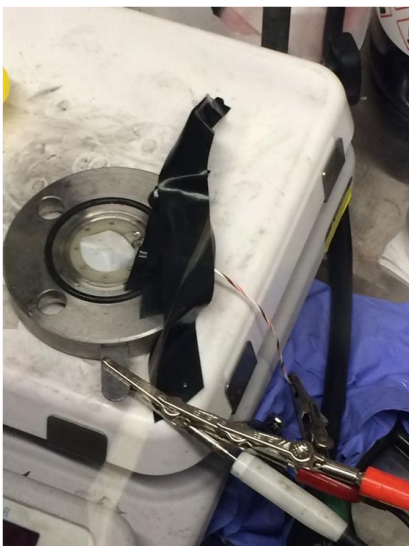
Figure 4.12: Picture of the working modified split-cell design. All subsequent tests on \text{T-LiFe}_{0.9}\text{Co}_{0.1}\text{O}_2 were performed with on a modified split-cell set up pressed with a weight glass vile.
