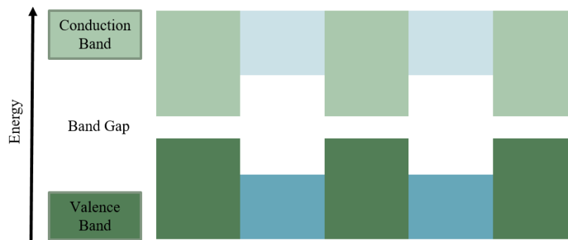
Figure 1.3 Schematic diagram of a band diagram resulting from a quantum-well superlattice.
