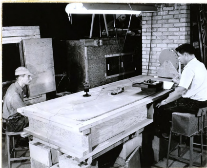
Fig. 10. View of apparatus used for measuring potential distributions along a vertical diameter of a charged dust cloud.
