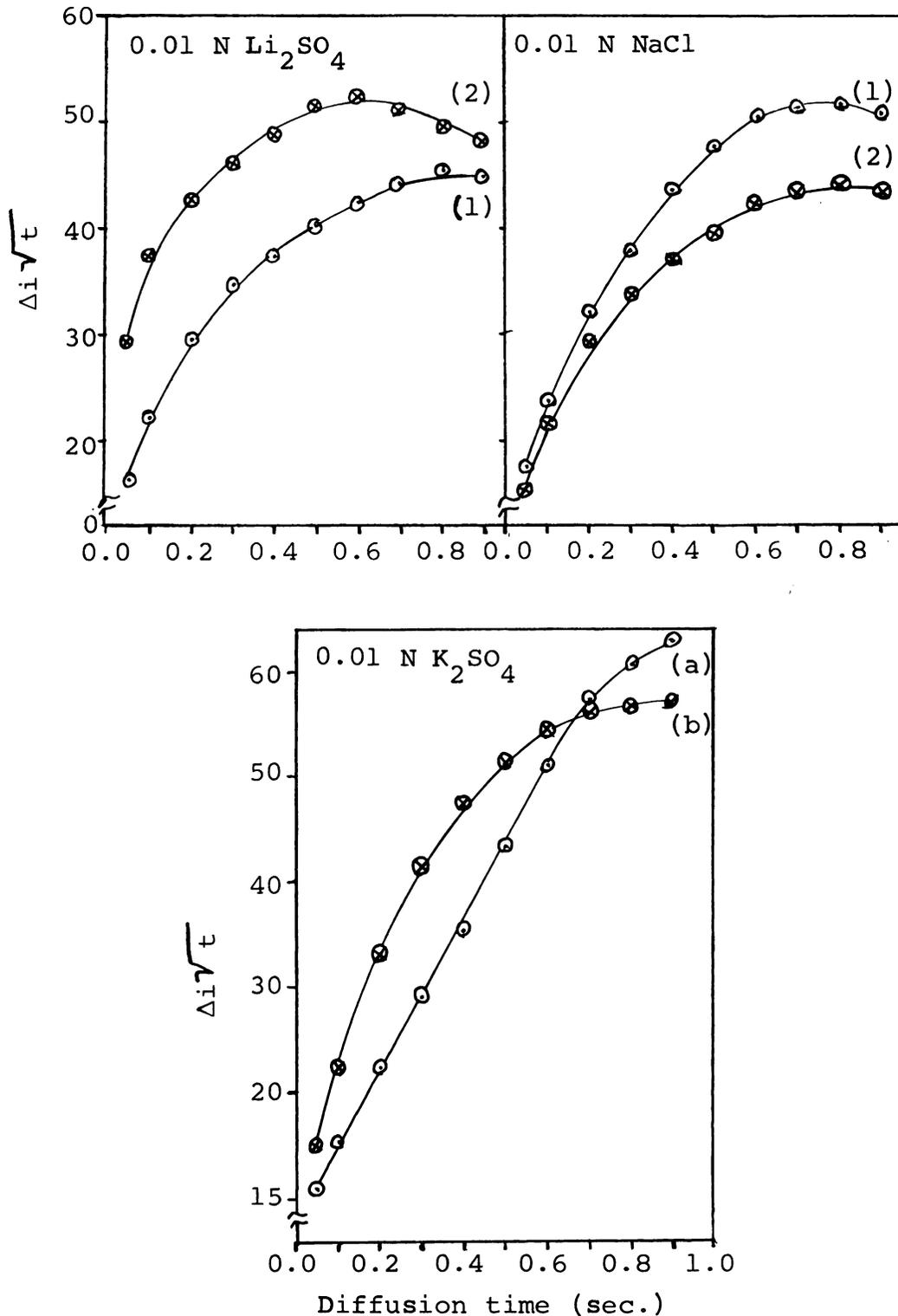
Figure 20. Variations in  $\Delta i\sqrt{t}$  from 0.01 N  $\text{Li}_2\text{SO}_4$ , NaCl and  $\text{K}_2\text{SO}_4$  using different electrode treatments.
