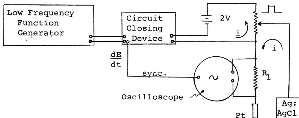
Figure 5. Simplified schematic diagram of the oscillographic polarograph that applies a direct current square wave to the electrodes. A detailed schematic appears on page 35.
