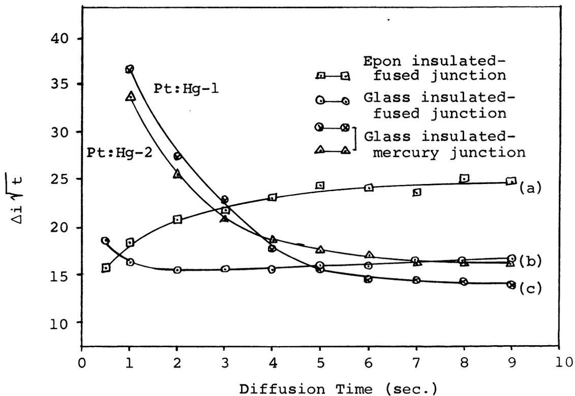
Figure 13. Influence of electrode type on  $\Delta i \sqrt{t}$ .
