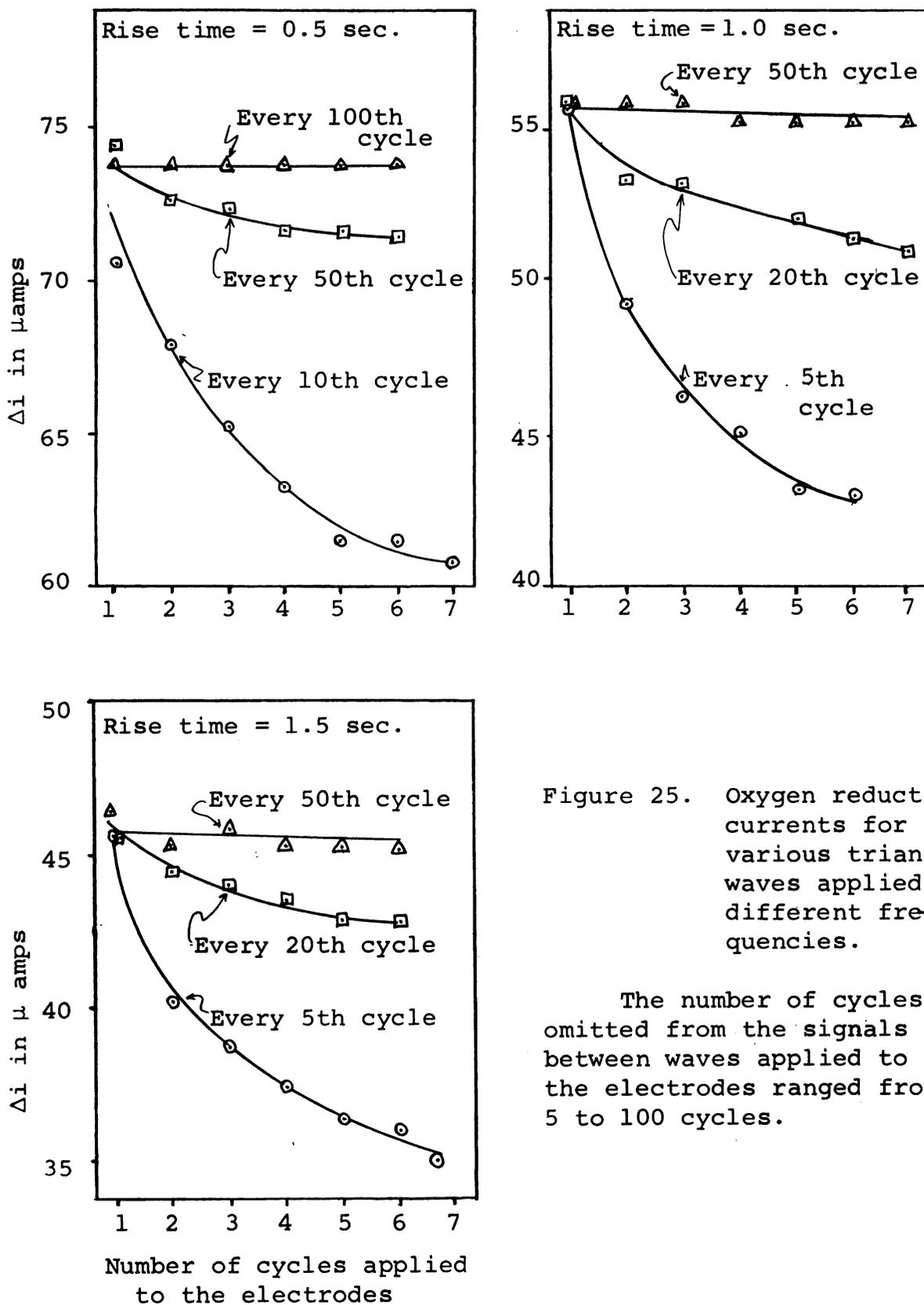
Figure 25. Oxygen reduction currents for various triangular waves applied at different frequencies.
