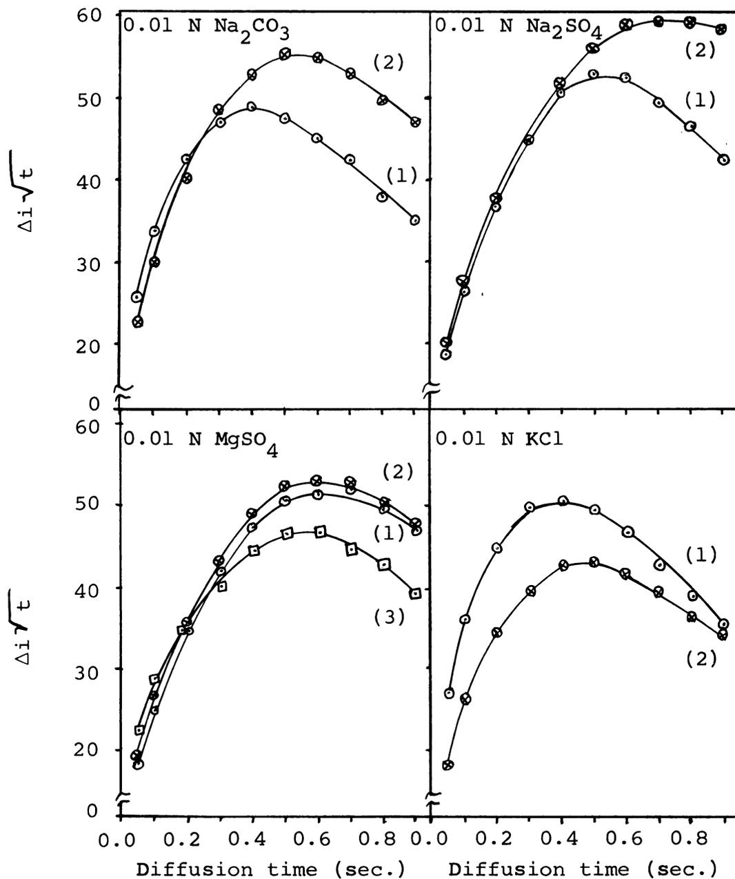
Figure 19. Variation in  $\Delta i\sqrt{t}$  from 0.01 N  $\text{Na}_2\text{CO}_3$ ,  $\text{Na}_2\text{SO}_4$ ,  $\text{MgSO}_4$  and KCl using different electrode treatments.
