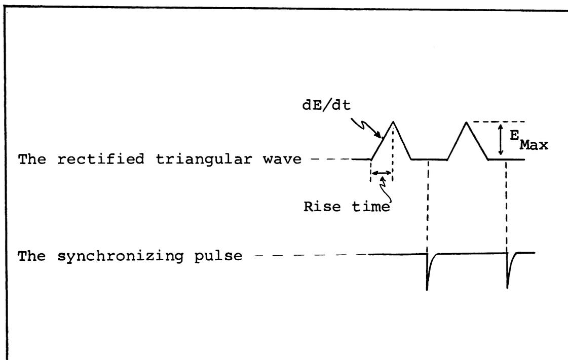
Figure 22: The wave forms from the function generator.
