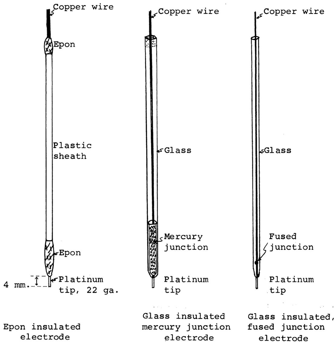
Figure 7. Diagram of three kinds of electrodes studied.
