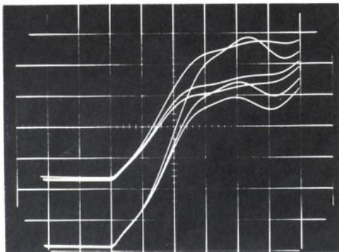
Figure 24. The current-time curves from three successive cycles of a triangular wave applied to an electrode.
