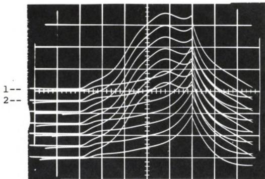
Figure 23. Polarograms recorded to obtain oxygen reduction currents.
