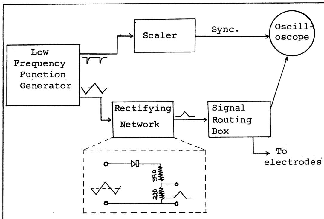
Figure 21. Simplified schematic diagram of the apparatus for applying a triangular wave to the electrodes and automatically presenting the polarogram on an oscilloscope.
