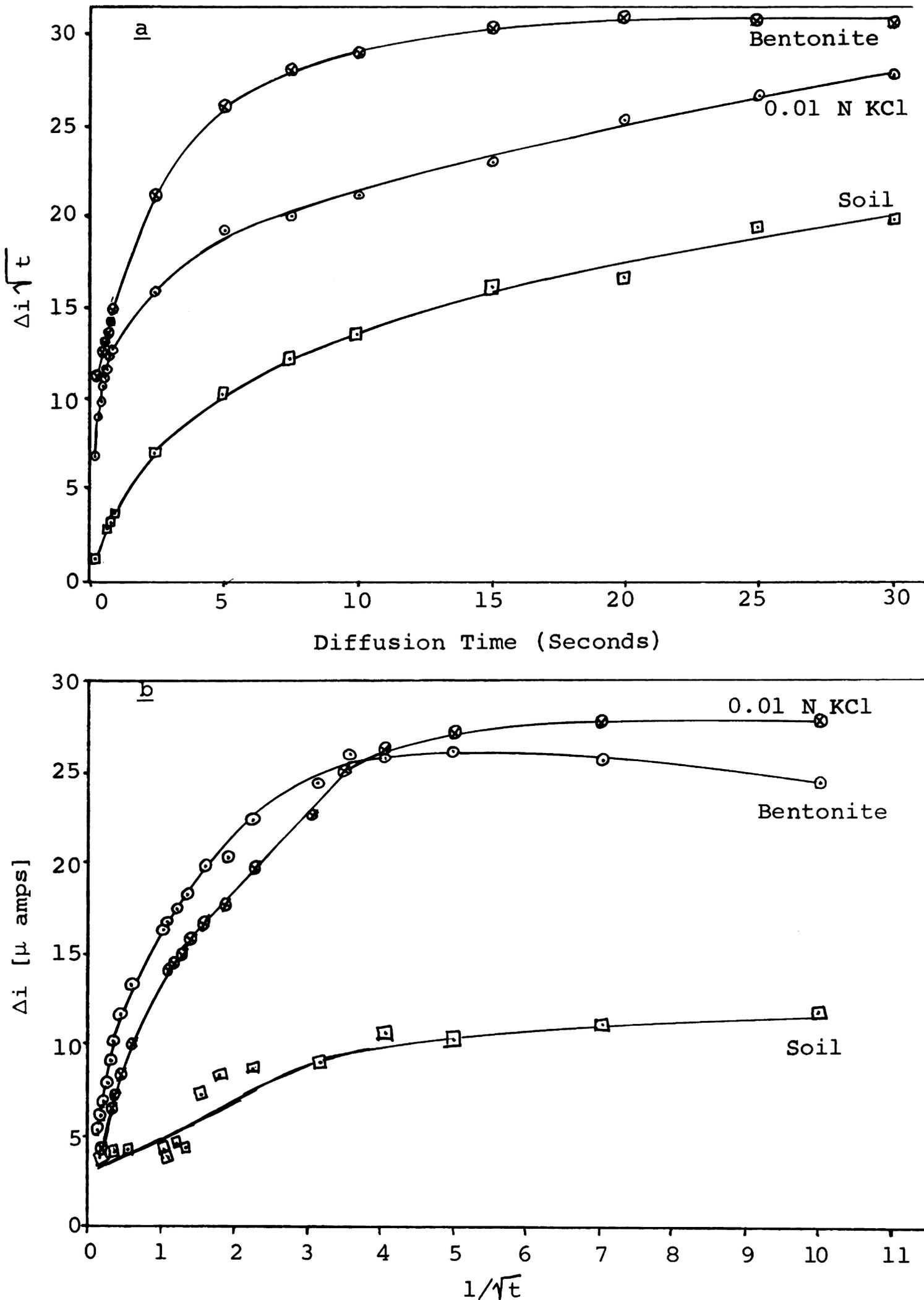
Figure 9. Tests for linear diffusion in the data of Tables 1, 2 and 3. Epon insulated electrodes were used at an applied voltage of -0.65 volt.
