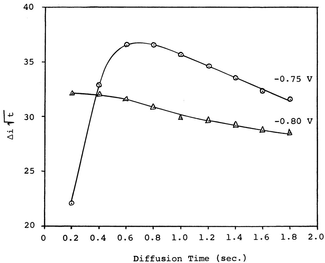
Figure 15. The influence of applied voltage on  $\Delta i \sqrt{t}$  for glass insulated electrodes.
