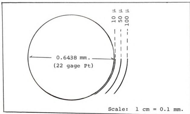
Figure 4. Diffusion shells of 10, 50 and 100 microns thickness drawn parallel to the surface of 22 ga. platinum wire (in cross section).
