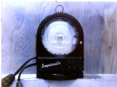
Figure 23. The recorder which kept an on-and-off record of the operation of the ventilating fans.
