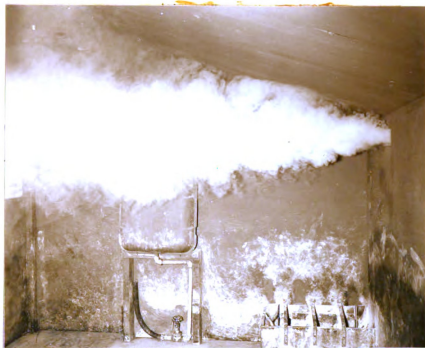
Figure 29. The distribution of the air as it enters the house through one of the air intakes in the rear wall.
