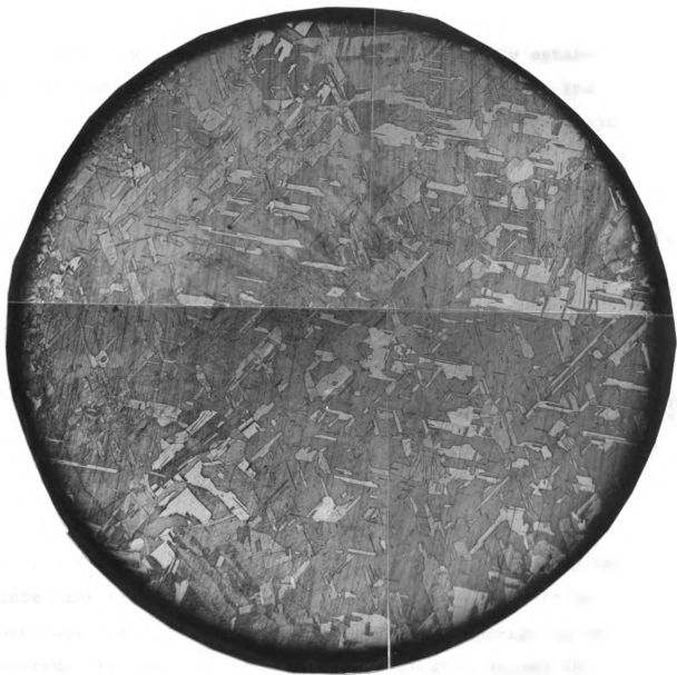
c) after annealing at 550° C
