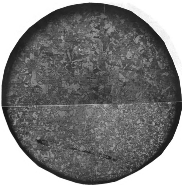
b) after annealing at 500° C
