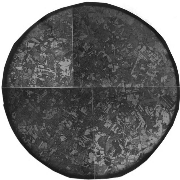
c) after annealing at 550°C
