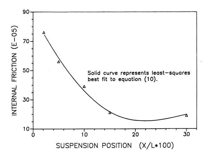
Figure 16. Measured internal friction as a function of suspension position (x/l \*100) for the alumina/SiC composite specimen HP160.
