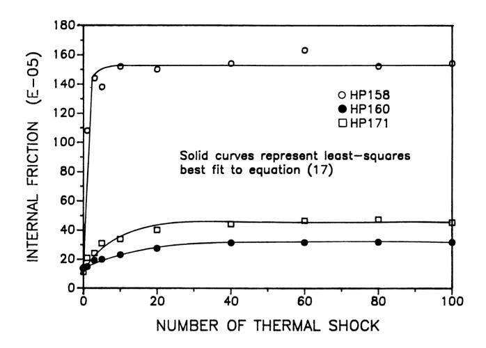
Figure 21a. Internal friction of the alumina/SiC composite specimens HP160 ( $\Delta T$ =270 degrees C), HP171 ( $\Delta T$ =310 degrees C) and HP158 ( $\Delta T$ =380 degrees C) as a function of thermal shock cycle.
