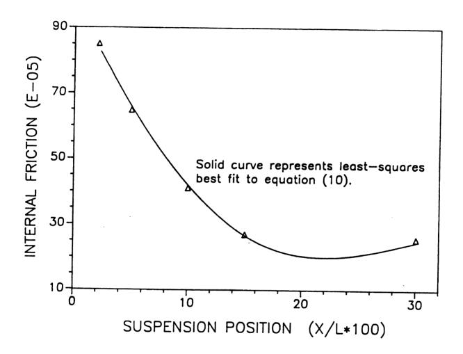
Figure 17. Measured internal friction as a function of suspension position (x/l \*100) for the alumina/SiC composite specimen HP171.
