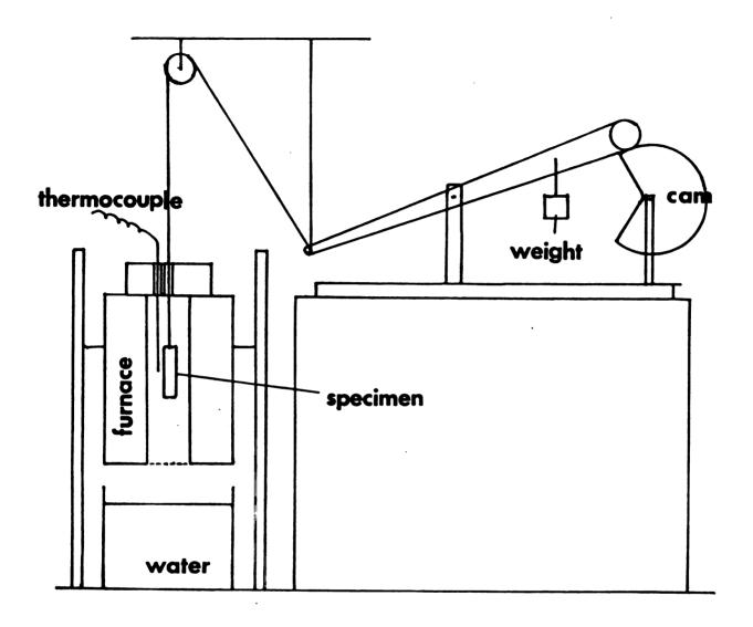
Figure 9. Schematic diagram of the thermal shock test apparatus.
