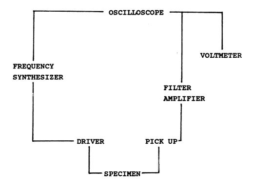
Figure 5. Outline of apparatus for measuring the elastic modulus (Dynamic resonance method).
