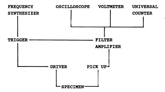
Figure 7. Internal friction apparatus diagram.
