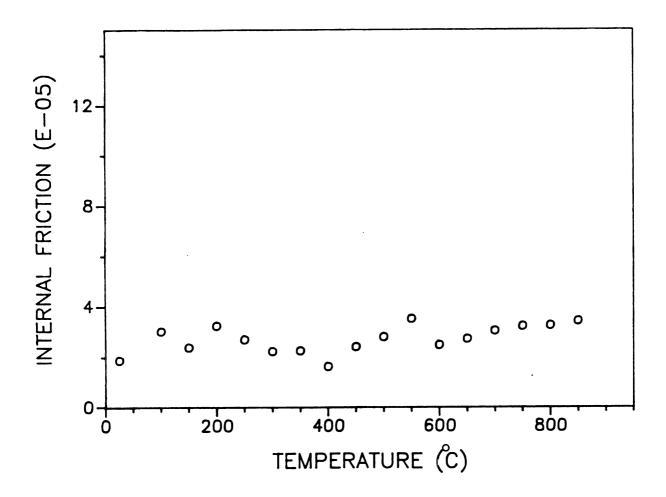
Figure 19. Internal friction of the alumina/SiC composite specimen HP171 as a function of temperature (Measurement performed prior to thermal shock treatment of specimen HP171).
