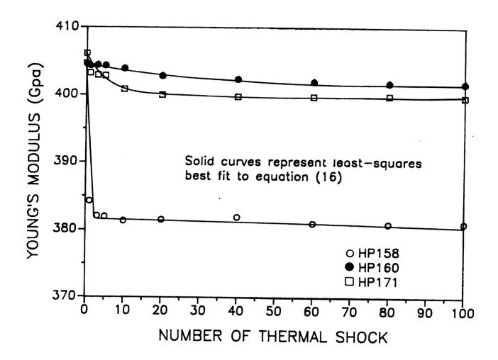
Figure 20a. Young's modulus of the alumina/SiC composite specimens HP160 ( $\Delta T$ =270 degrees C), HP171 ( $\Delta T$ =310 degrees C) and HP158 ( $\Delta T$ =380 degrees C) as a function of thermal shock cycle.
