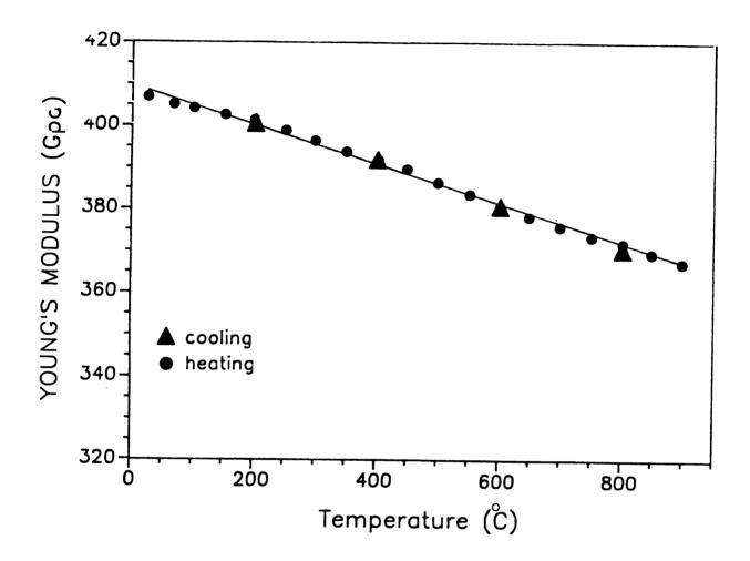
Figure 18. Young's modulus of the alumina/SiC composite specimen HP171 as a function of temperature (Measurements performed prior to thermal shock treatment of specimen HP171).
