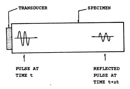
Figure 3. Schematic illustration of ultrasonic pulse method (After Norwick and Berry [13]).
