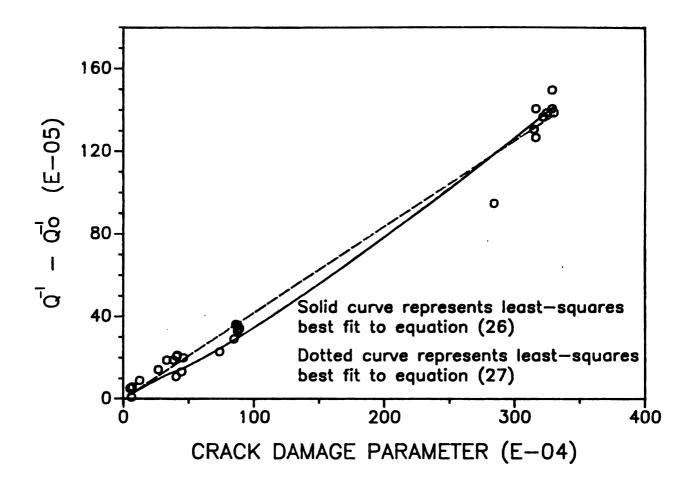
Figure 22. Internal friction change,  $\Delta Q^{-1}$ , as a function of crack damage parameter,  $\epsilon$ , for the SiC whisker/alumina composites.
