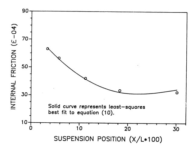
Figure 14. Measured internal friction as a function of suspension position (x/l \*100) for the polymer composite AU4-longitudinal.
