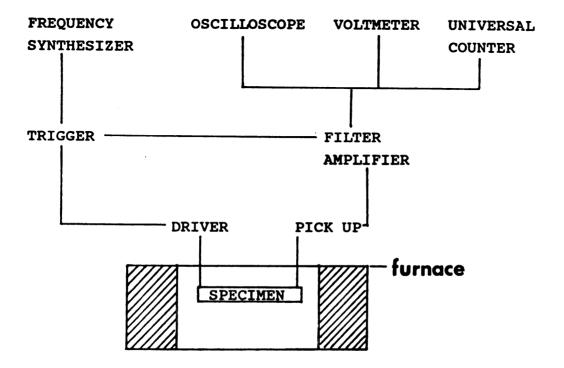
Figure 8. Schematic diagram of the elevated temperature elasticity and internal friction measurement apparatus.
