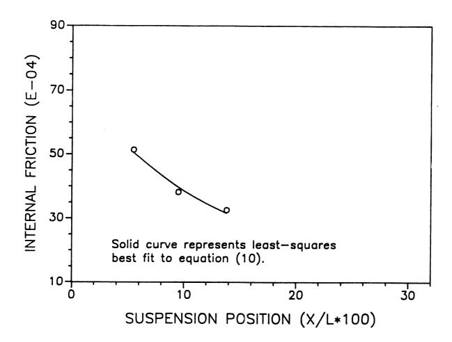
Figure 13. Measured internal friction as a function of suspension position (x/l \* 100) for the polymer composite specimen AS4C-longitudinal.
