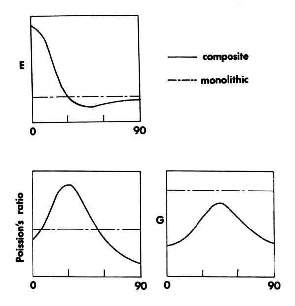
Figure 10. Variation of elastic moduli of a fiber composite and a monolithic material with the angle of reinforcement (After Meyer and Chawla [21]).
