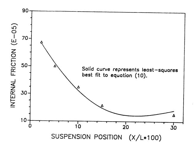
Figure 15. Measured internal friction as a function of suspension position (x/l \*100) for the alumina/SiC composite specimen HP158.
