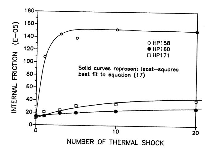
Figure 21b. Internal friction of the alumina/SiC composites HP158, HP160, and HP171 versus thermal shock number. Data in this figure is a subset (namely, the first twenty thermal shocks) of the data presented in figure 21a. Note that even for n small, equation (17) fits the data relatively well.
