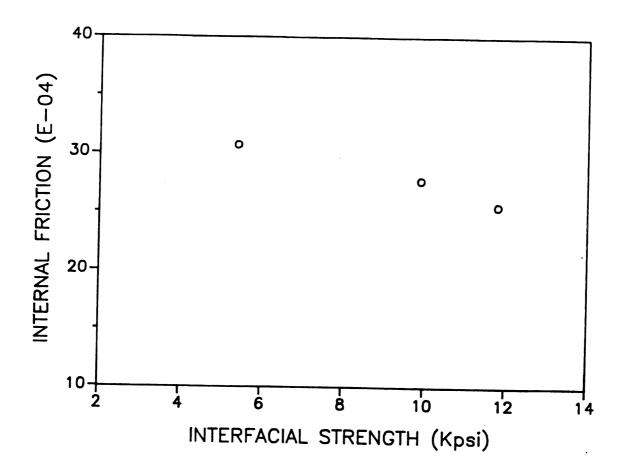
Figure 11. Internal friction of polymer composites as a function of interfacial shear strength.
