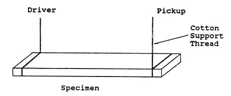
Figure 6. Illustration of method of coupling accoustic energy.
