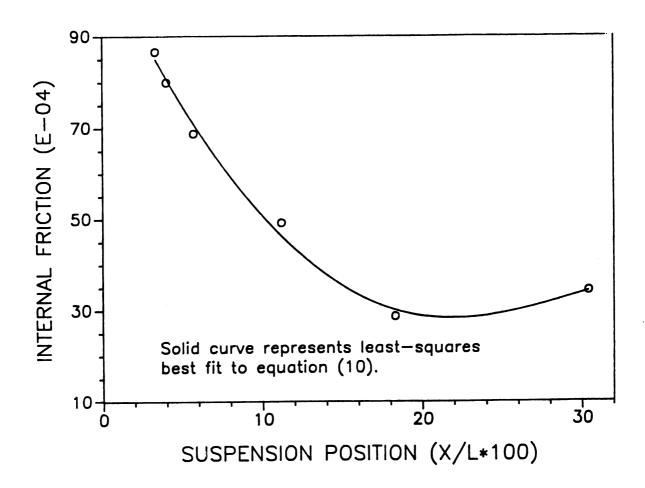
Figure 12. Measured internal friction as a function of suspension position (x/1 \* 100) for the polymer composite specimen AS4-longitudinal.
