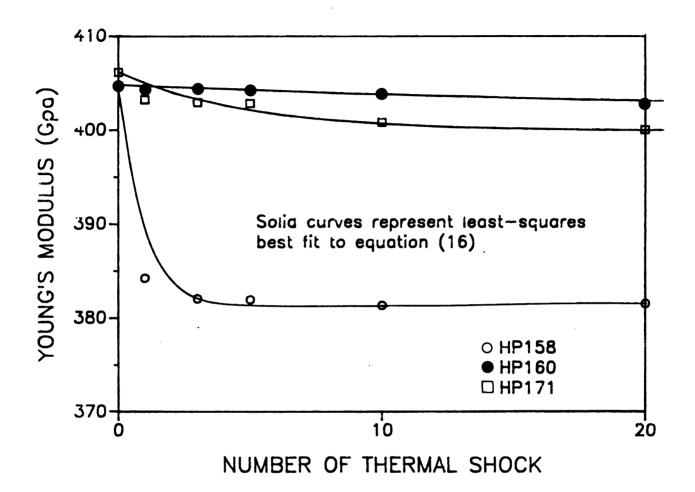
Figure 20b. Young's modulus of the alumina/SiC composites HP158, HP160, and HP171 versus thermal shock number. Data in this figure is a subset (namely, the first twenty thermal shocks) of the data presented in figure 20a. Note that even for n small, equation (16) fits the data well.
