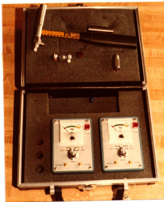
Figure 4-2 Typical Hammer Kit for Modal Analysis.
