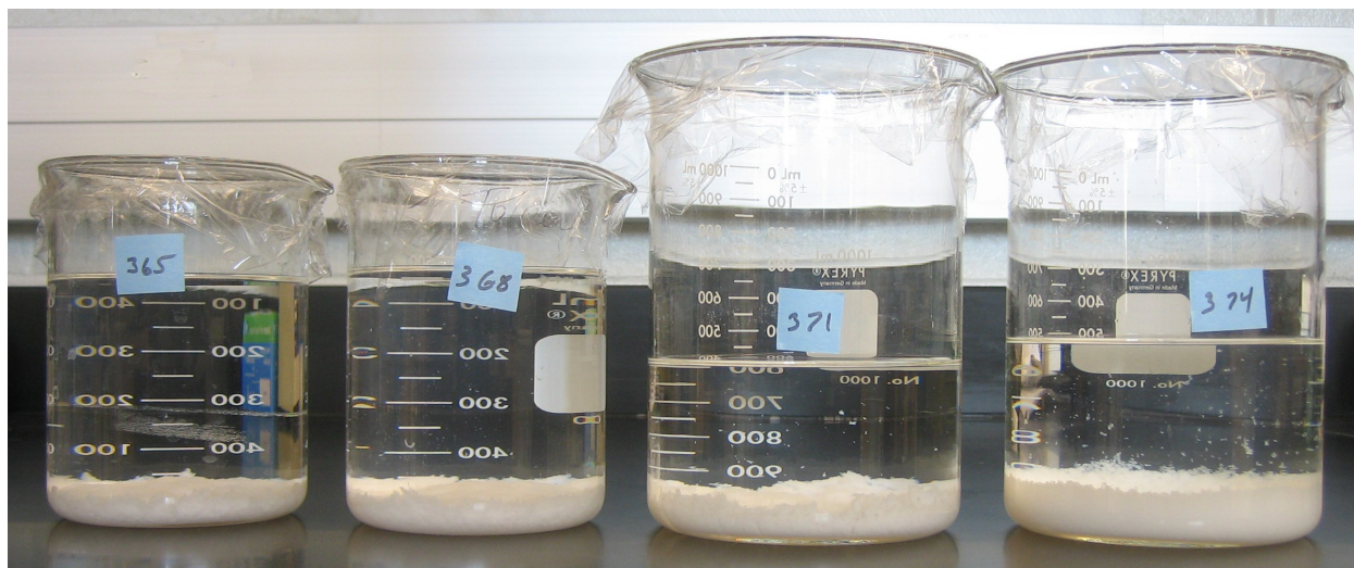
(b) Precipitates from 50 mg/mL 393 kD polystyrene solutions with and without crosslinked polystyrene nanoparticles. All supernatants are clear.
