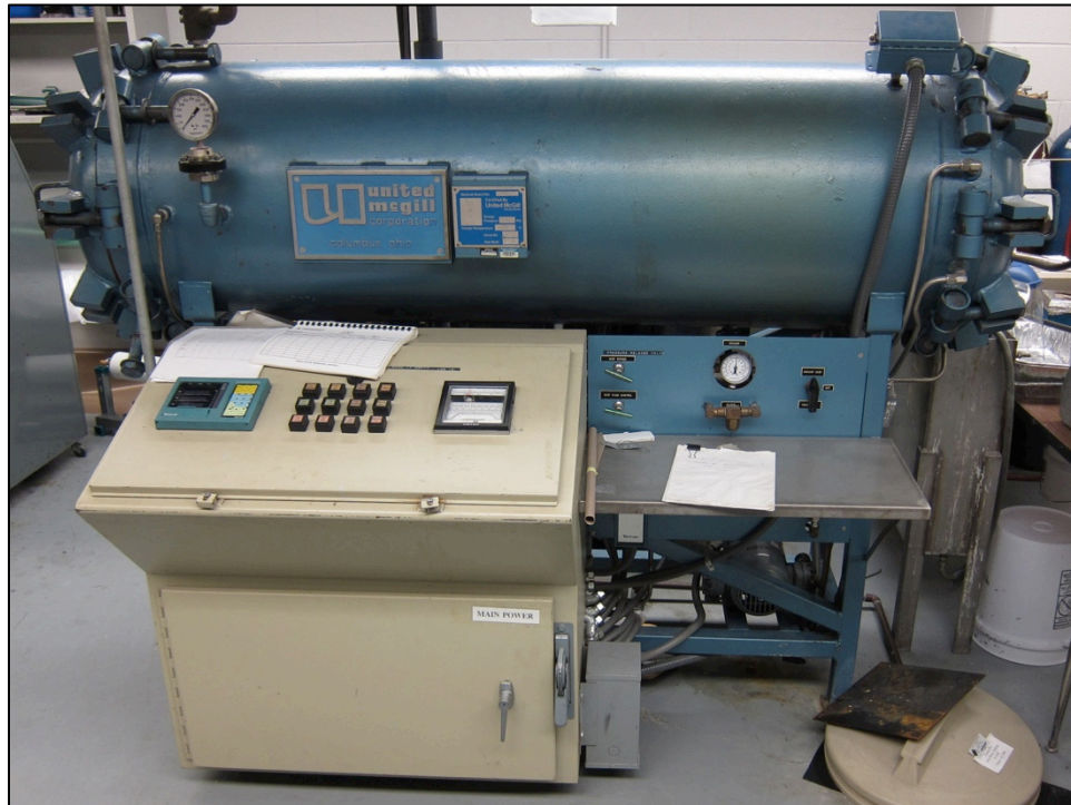
Figure 3.5: United McGill Minibonder autoclave
