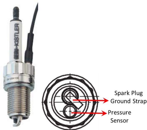
**Figure 3.2:** Front- and bottom-views of the spark plug combined with pressure sensor for pre-chamber measurements.
