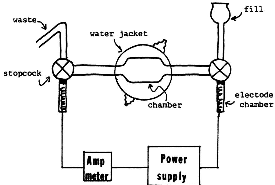
Figure 3. Diagram of chamber and electrode circuit.
