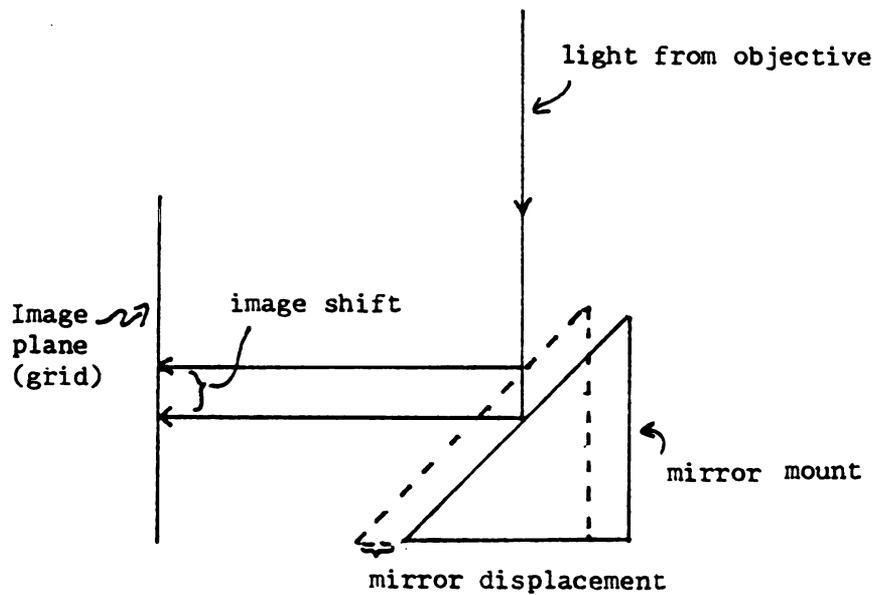
Figure 1. Diagram of mirror movement.
