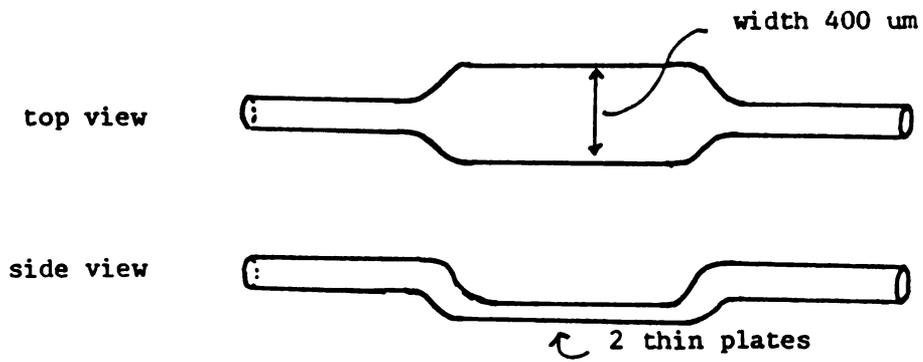
Figure 2. Diagram of measuring chamber.
