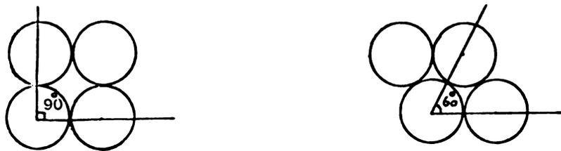
Figure 2.3.--The Angle of Intersection of the Sets of Rows in the Layer.
