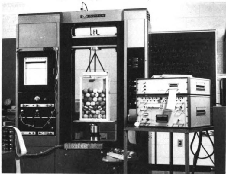
Figure 7.9-- A Complete Set-Up of the Simulated Force Distribution Experiment of Two Dimensional Rhombohedral Arrangement of the Rubber Balls
