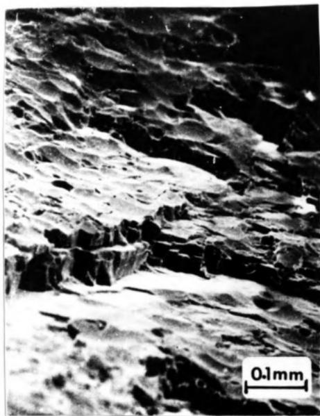
Fig. 46. A scanning electron micrograph of  $\text{CaF}_2$  eroded by 0.25 mm glass beads impacting the  $\{111\}$  at a velocity of 75 m/s.
