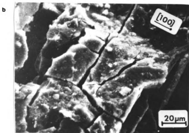
Fig. 50. A scanning electron micrograph of KCl eroded by 0.25 mm glass beads impacting the {001} at a velocity of 75 m/s.
