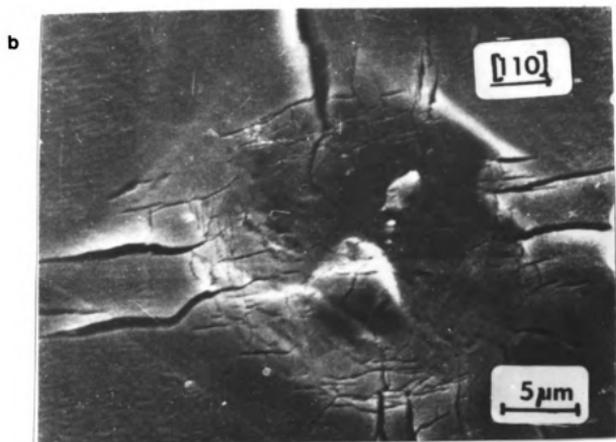
Fig. 14. Formation and reorientation of chips during impact.
