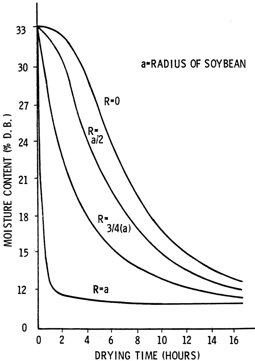
Figure 3.6. Moisture Content Distribution of the Soybean Model at Different Radii for the Whole Drying Period ( $z=0$ )
