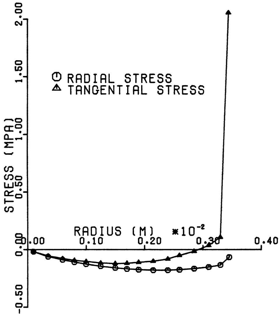
Figure 5.3. Simulated Radial and Tangential Stresses at the Time Tangential Stress Reaches its Maximum (One Hour)
