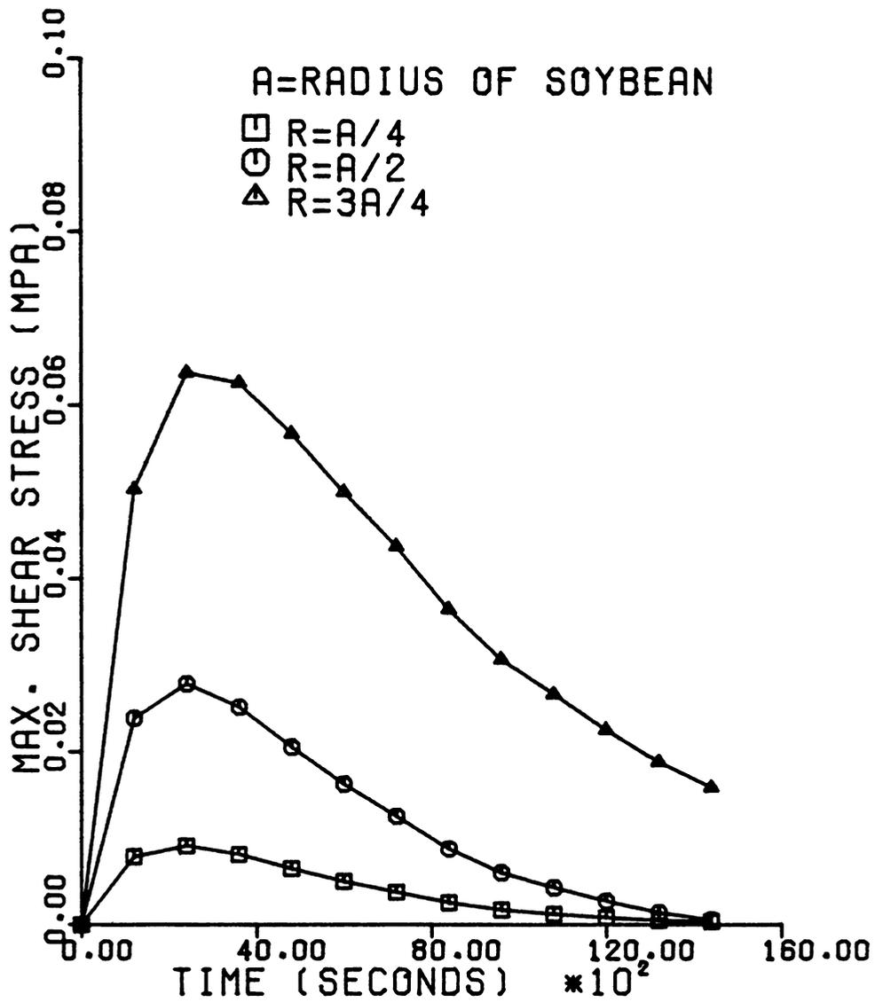
Figure 5.1. Simulated Maximum Shear Stress at Different Radii Inside the Soybean Model
