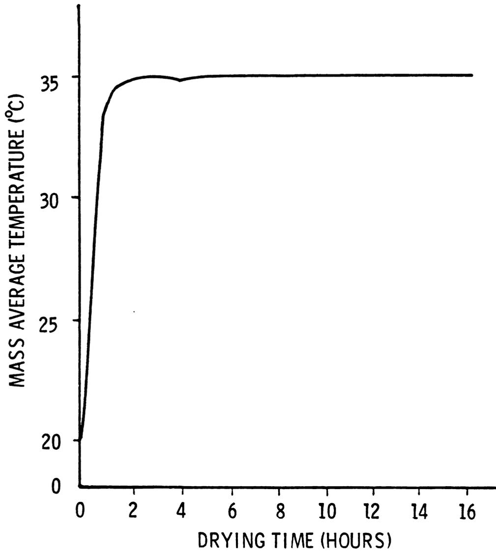
Figure 3.5. Simulated Mass Average Temperature of the Soybean Model vs. Time
