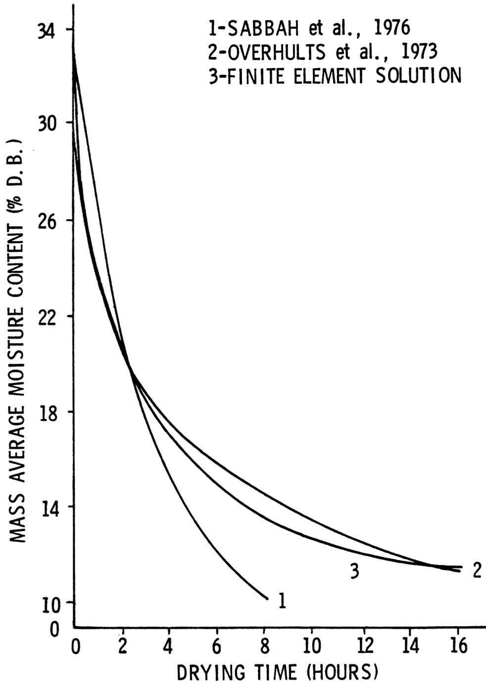
Figure 3.4. Drying Curve for the Soybean Model Compared with Experimental Results
