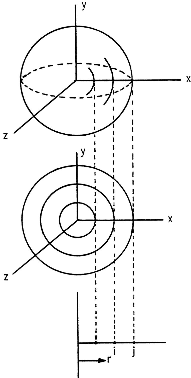
Figure 4.3. Radially Symmetric Line Elements and Corresponding Concentric Shells
