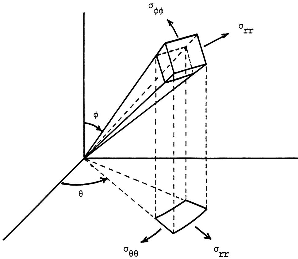
Figure 4.2. Stresses in Radially Symmetric Problems
