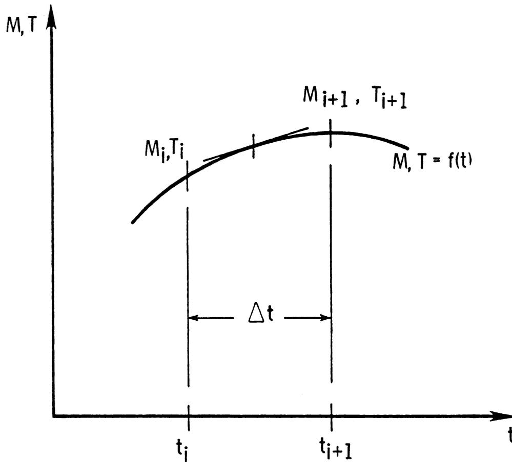
Figure 3.2. Numerical Determination of the First Derivatives of  $\{M\}$  and  $\{T\}$
