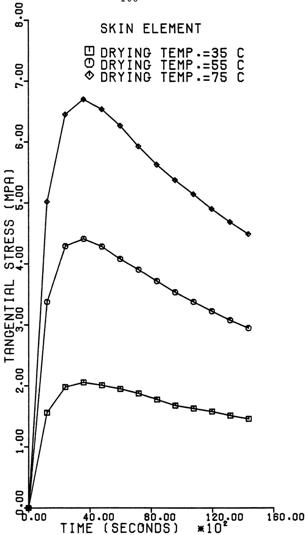
Figure 5.5. Simulated Tangential Stress at the Surface as Affected by Drying Temperature
