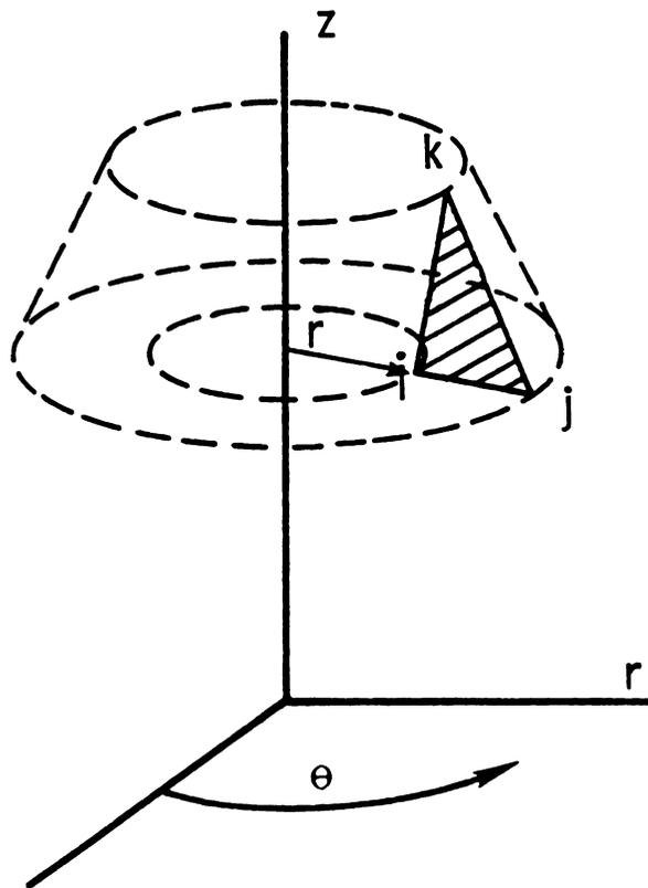
Figure 3.1. Simplex Triangular Axisymmetric Elements
