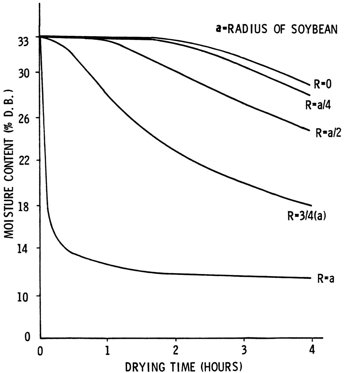
Figure 3.7. Distribution of the Soybean Moisture Content at Different Radii for the First Four Hours of Drying
