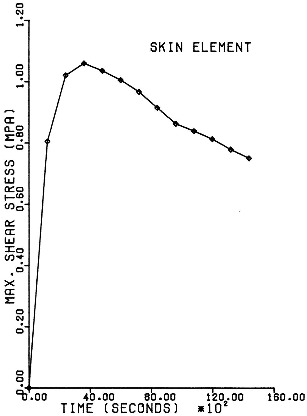
Figure 5.2. Simulated Maximum Shear Stress at the Surface
