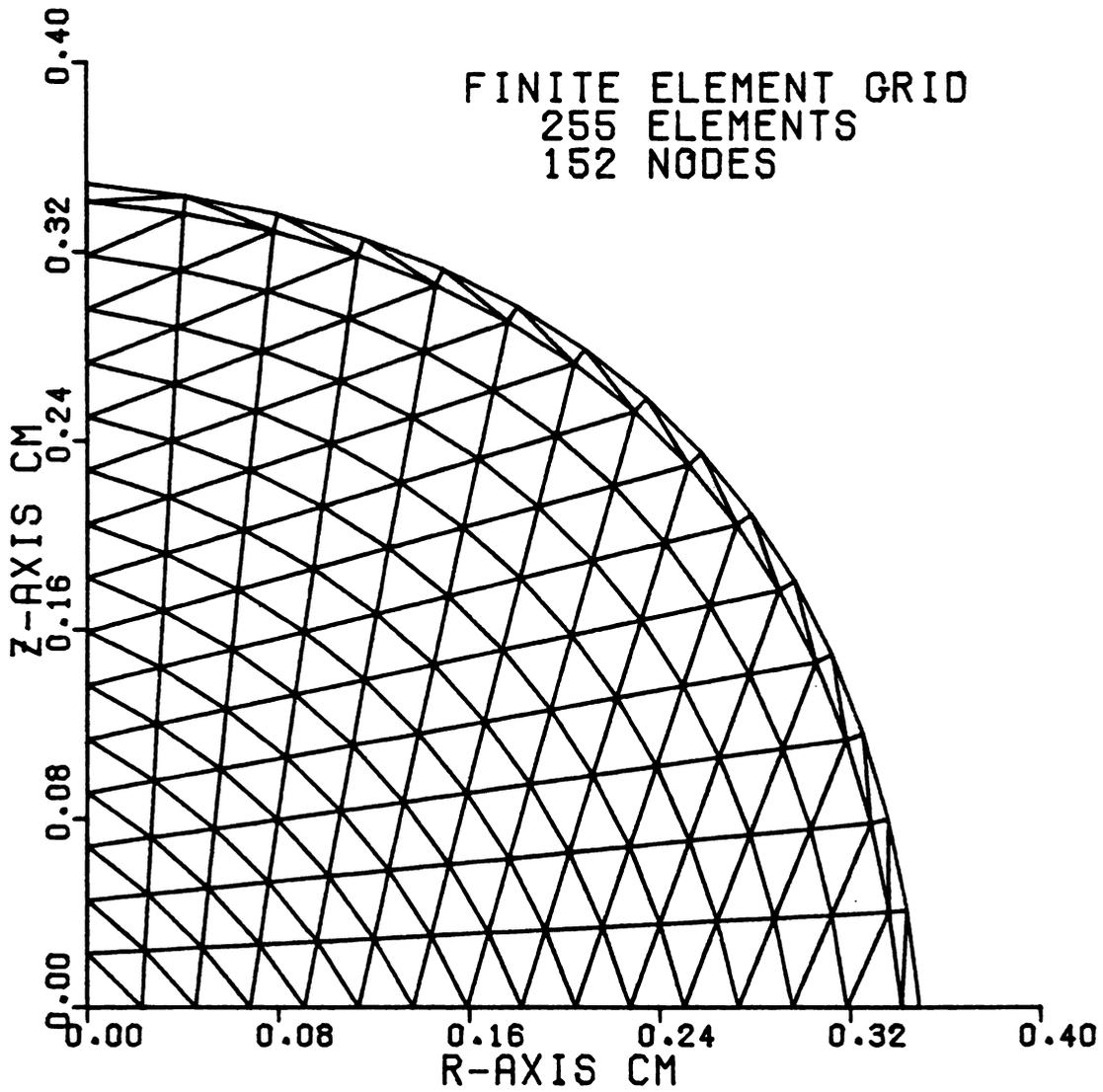
Figure 3.3 The Two-Dimensional Axisymmetric Finite Element Grid with Simplex Triangular Elements
