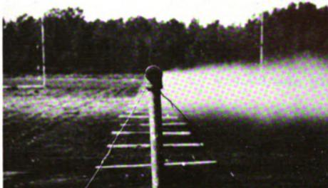
FIGURE 6.4.2.1.--Operational spray line for small water droplets.
