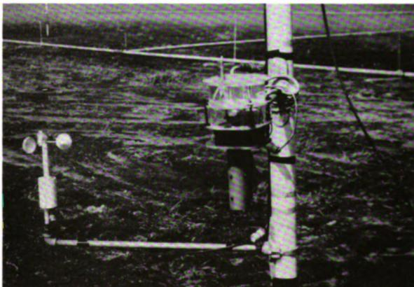
FIGURE 5.3.1.5.--A close up view of the anemometer and a psychrometer arrangement.
