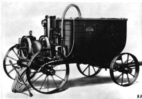
1925. This model had a 5\frac{1}{2} g.p.m. pump and a 2\frac{1}{2} H.P. engine for 250 lbs. pressure. The tank had 100 gallons capacity.
