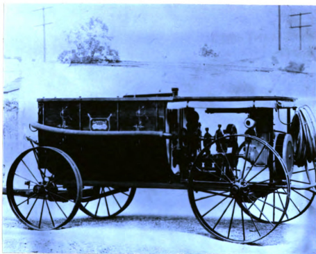
1924. Using a light weight 6 H.P. engine for power, the Triplex Pump now delivered 12 g.p.m. at 300 - 350 lbs. pressure.
