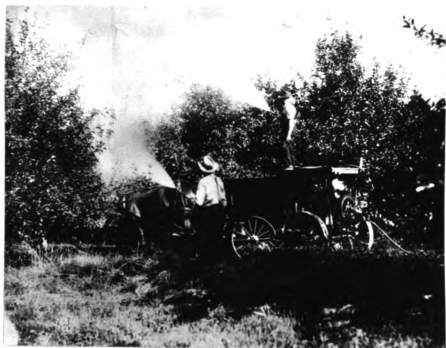
1918. Powered by a 3 H.P. engine, the Bean Triplex Pump now delivers 8 g.p.m. at 250 lbs. pressure. The tank has been increased to 200 gallons and spray guns which came into general use that year have replaced the long bamboo rods and small nozzles.
