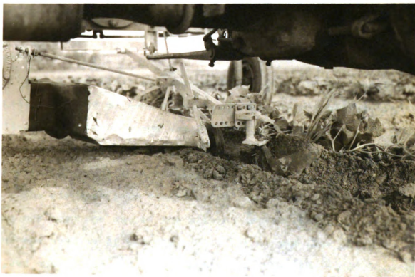
Figure 8. Pneumatic vine trainer. Note air distributor, gage wheel, and shovel.
