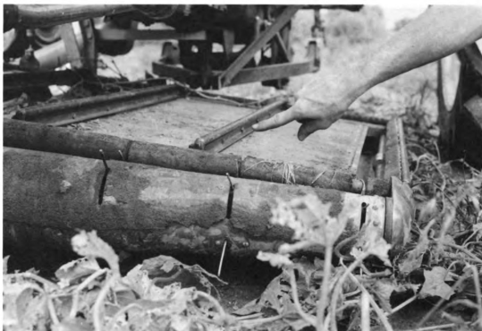
Figure 31. Roller flights installed on the separating bed during the later part of the testing season.
