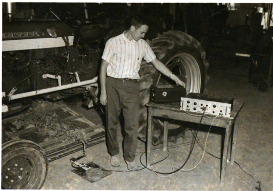
Figure 20. The author observing the strain gage transducer and recording equipment.
