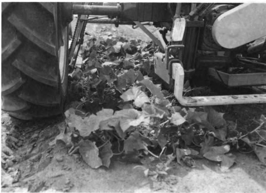
Figure 32. Position of vines after leaving the separating bed.
