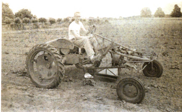
Figure 7. Pneumatic vine trainer mounted on Allis Chalmers Model G tractor.
