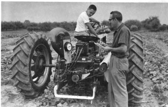
Figure 18. The author and Dr. Buchele observing the operation of the torque meter under field conditions.
