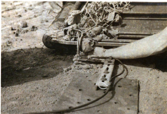
Figure 19. Strain gage transducer used in measuring the forces on the vine by the separating bed.
