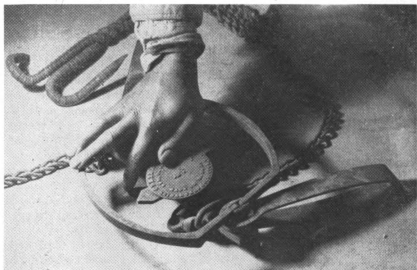
Figure 6. No. 4 1/2 wolf trap with longer chain and larger toggle, for use on black bears. Man's hand indicates how a bear could prevent a trap from closing on its foot.
