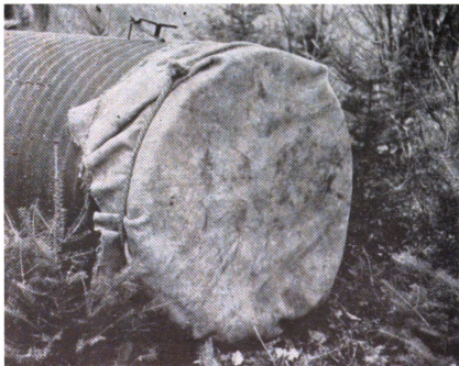
Figure 10. Canvas sealing grid back of sprung culvert trap to prevent escape of ether.
