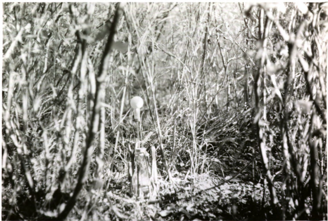
Plate 2. Set up of the Livingston atmometer in a Swamp Shrubs stand. Bulb was approximately 18 inches above the ground.
