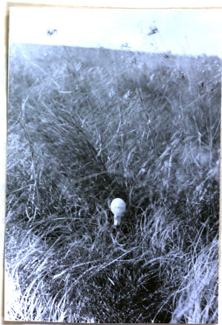
Plate 1. Set up of the Livingston atmometer in a Marsh stand. Inflorescences of Scirpus cyperinus can be seen on the upper part of the photograph. Bulb was approximately 18 inches above the ground.
