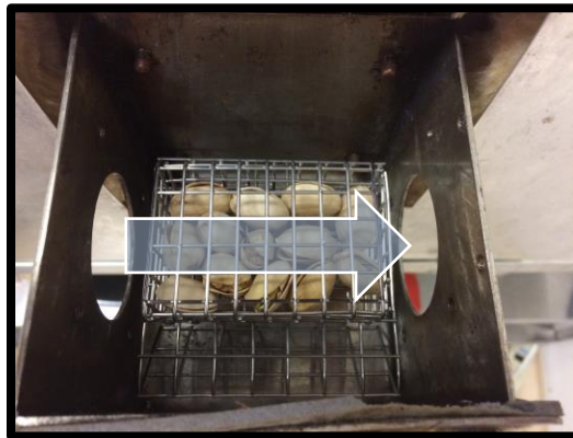
Figure 10. Photo of the pistachios in the sample rack in the heating chamber. Arrow indicates direction of flow.
