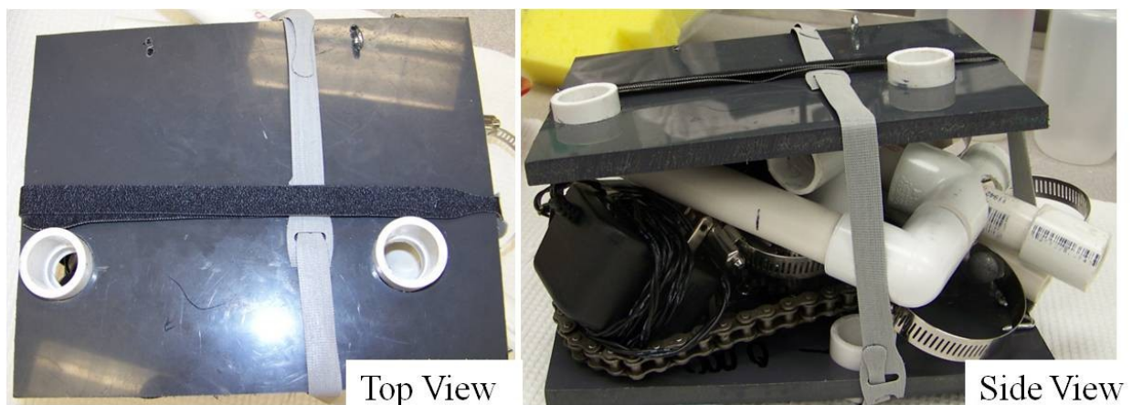
Figure 9.3: The lab designed, portable, 200 mL bottle rotator used for the 40 minute rotation as the EAMNPs capture the bacteria in its compacted transport formation.
