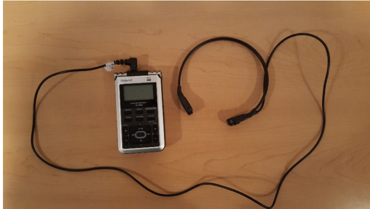
Figure 1: VoxLog collar and Roland recorder.
