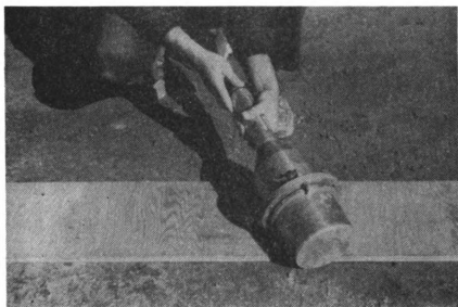
Figure 5-2. Roll-A-Meter for Volumetric Air Tests
