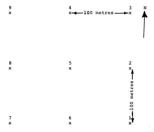
Figure 14: Layout of a Cluster of 9 Center Plots
