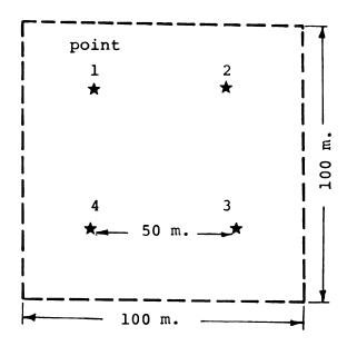
Figure 9: Wedge Prism Points at each Grid Location in Wheeler's Method
