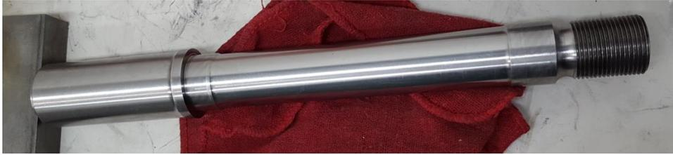
Figure 63 lower bearing housing main shaft
