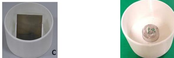
Figure 59 sabot with Ti blade shaped projectile (left) and another sabot with Al cylindrical projectile for instrumented target testing (right)
