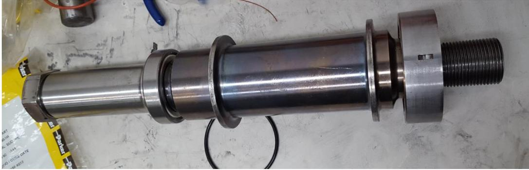
Figure 65 aft bearing carrier installation
