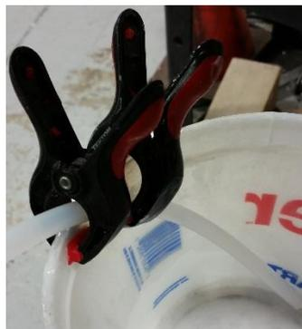
Figure 83 tube positioned for infusion
