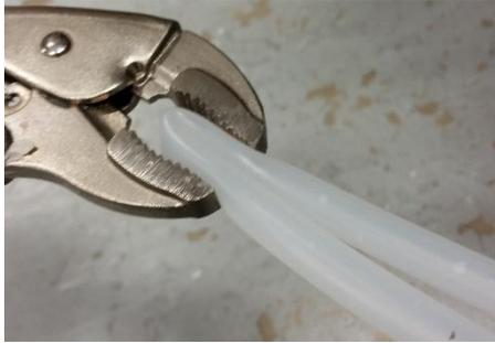
Figure 84 a method to kink tube when finished with resin
