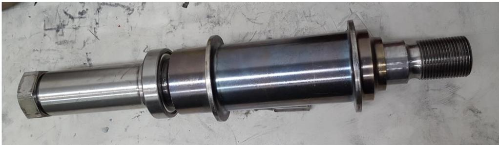
Figure 64 compression tube and forward bearing installation
