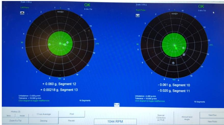
Figure 71 EasyBalance software results showing acceptable balance for both right and left planes
