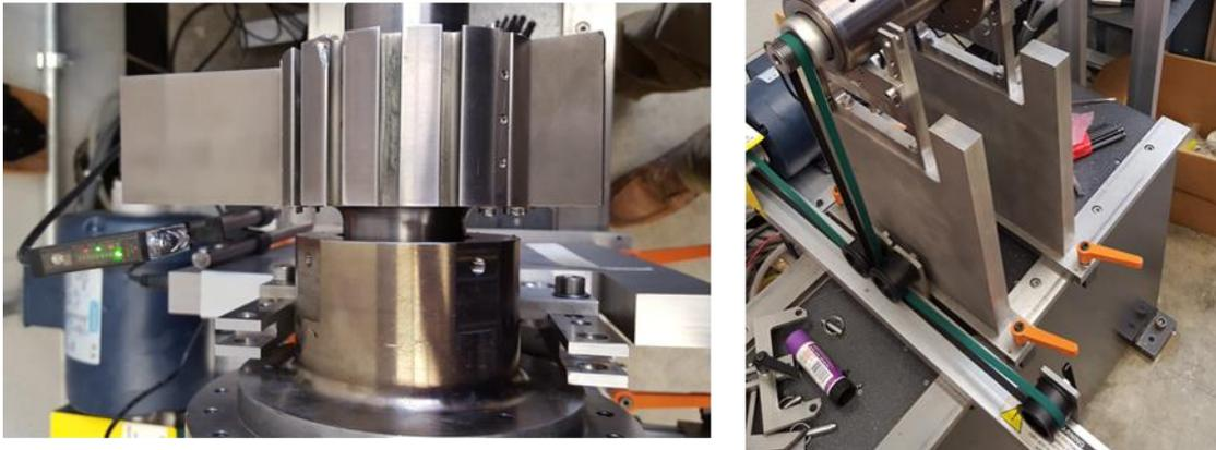
Figure 69 balance hardware laser speed pickup setup left and operating balance rig (right) The aft end of the shaft is driven by belt from the balance machine motor. The motor speed is adjusted so that the shaft spins approximately 1/30<sup>th</sup> of testing speed or 1000 RPM. Figure 69 right shows the operating balancing rig.
