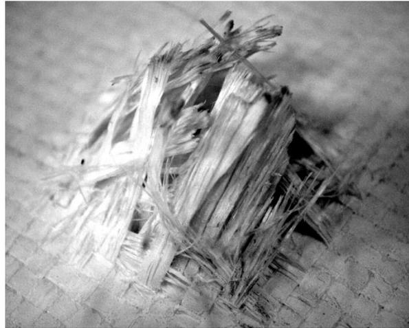
Figure 30 the back side of the composite panel from IT\_12, 6-ply panel tested at 458m/s: dry fiber tows are protruded and form a hut shaped sub-structure.
