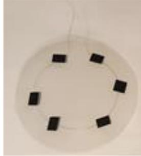
Figure 60 in-house manufactured poppet valve with Nichrome wire taped with same diameter as ID of barrel
