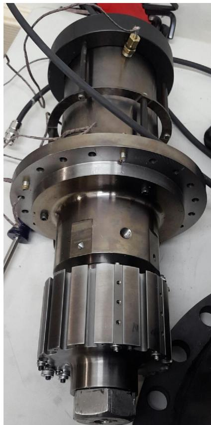
Figure 62 assembled inner bearing housing mocked up for temperature monitoring of forward and aft bearing
