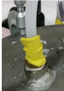
Figure 82 depiction of high temp tacky tape used to seal hose connections
