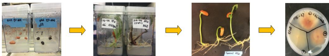
Figure 1.2 Diagram of Magenta box lab test showing growth medium, plants at harvest stage, harvested plants for rating and re-isolated Fusarium strains.
