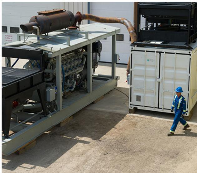
Figure 1.3: The E1 thermoelectric generator from Alphabet Energy. On the left is a large diesel generator, with the exhaust connected to the E1 TEG on the right.[1]
