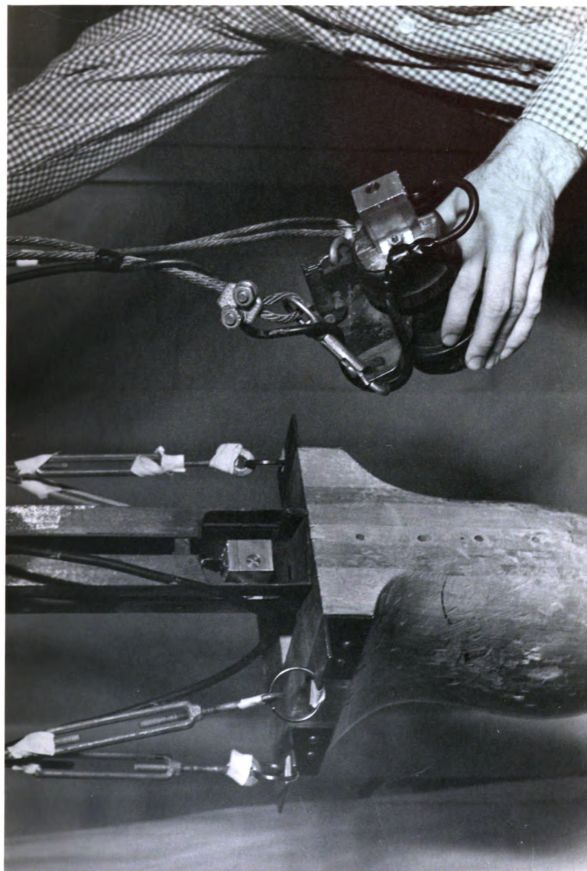
Fig. 64. Wooden Head, Insert with Accelerometer and Striking Pendulum with Accelerometer
