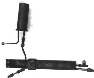
Figure 5.--Photograph of gasification reactor.
