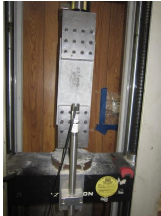
Figure 5.6 Ferrocement tension test setup
