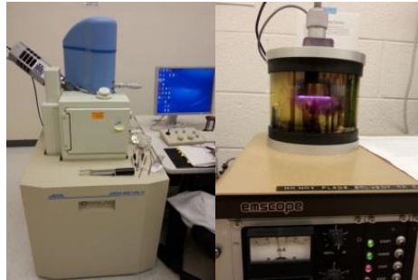
Figure 2.11 The scanning electron microscope (left) and the Emscope Sputter Coater analyzer (right) used in the project
