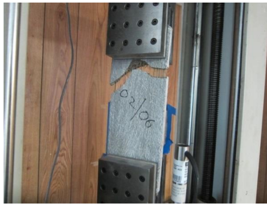
Figure 5.11 Failure of the first-generation ferrocement specimens with formation and growth of a single crack
