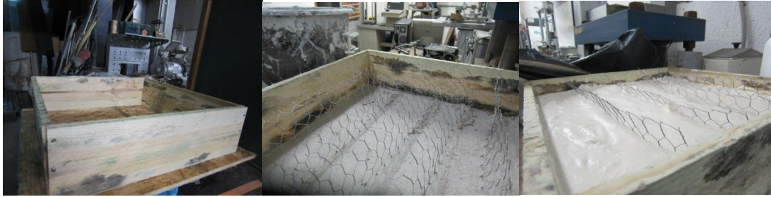
Figure 8.19 Production of the square sandwich composite component for performance of diagonal compression tests
