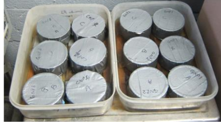
Figure 6.13 Sorption test specimens with one surface exposed to water
