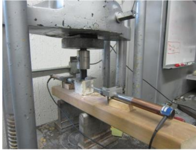
Figure 6.9 Compression testing of cube specimens with instrumentation for measurement of longitudinal force and deformation as well as transverse deformation
