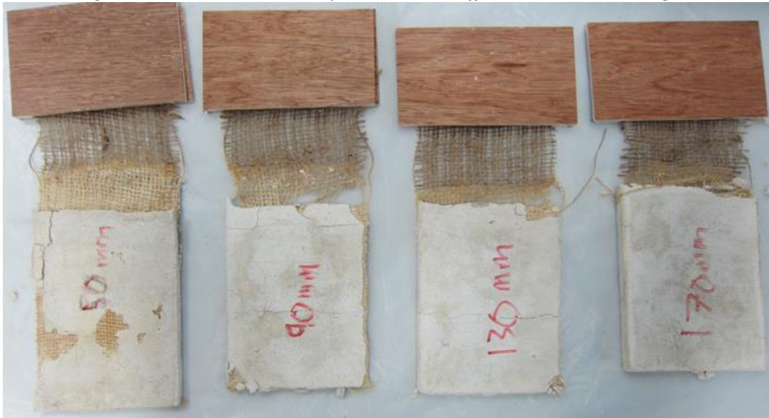
Figure 5.21 Failed bond test specimens with different embedment lengths
