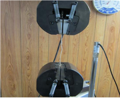
Figure 3.10 The single yarn tension test setup
