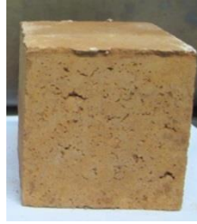
Figure 2.25 An alkali-activated laterite clay cube specimen.
