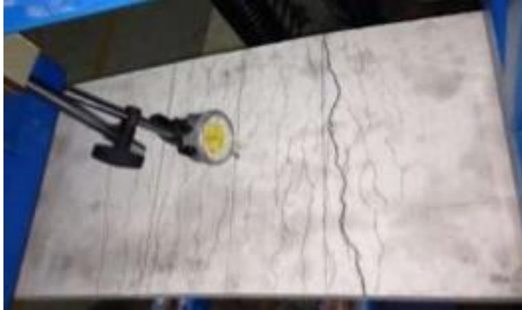
Figure 5.1 Multiple cracking of the tension face of a ferrocement panel under flexural loading
