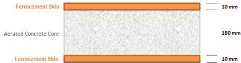
Figure 4.15 Preliminary thicknesses of the indigenous sandwich composite constituents
