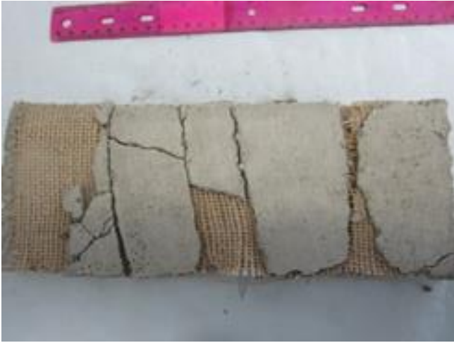
Figure 5.15 Delamination of the mortar coating on the outer layer of the 'Jute 1' burlap with fine opening size
