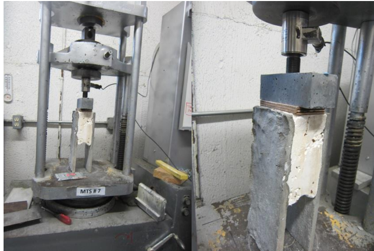
Figure 8.5 Interfacial shear test setup
