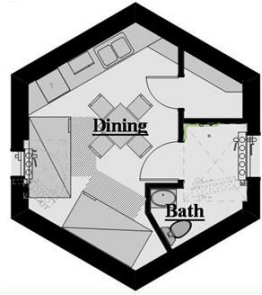
Figure 4.11 A single unit of the beehive shelter
