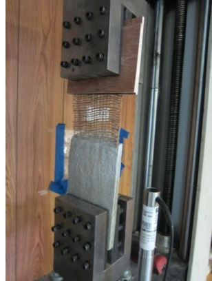
Figure 5.9 Pullout test setup
