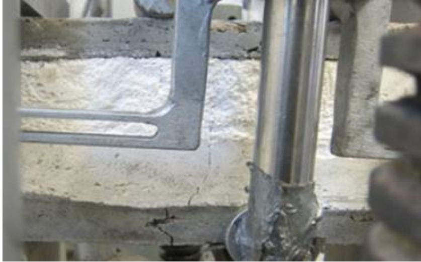
(a) Cracking of the aerated concrete core and tensile skin
