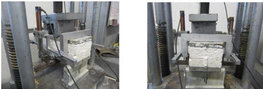
Figure 7.2 Sandwich composite flexure test setup
