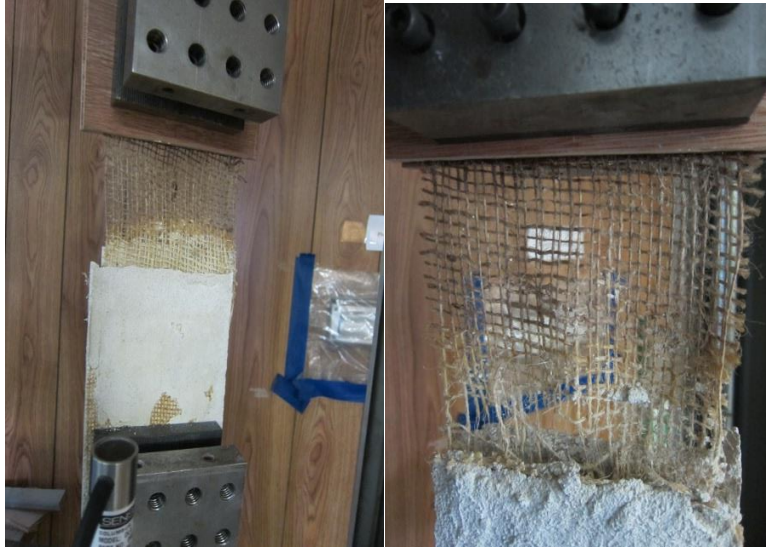
(a) Pullout of fabric with 50 mm embedment length
