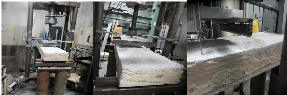
Figure 8.11 Long-span indigenous sandwich composite panel test setup
