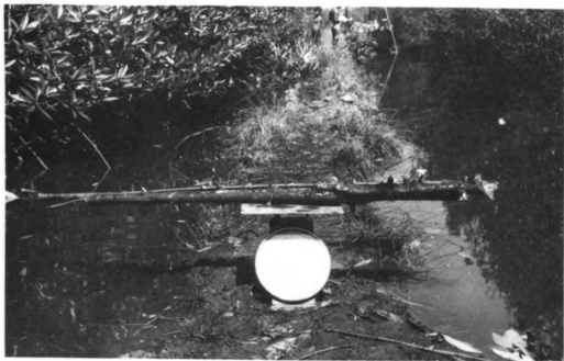
Figure 25. Field weighing a 2 m tree stem section.
