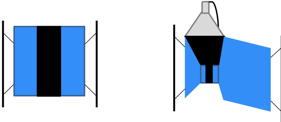
**Figure 2.3: The tsetse target and the trap.** The target (on the left) is two-dimensional device and usually applied with insecticide; The NG2G trap (on the right) is three dimensional with insecticides as an optional choice (Adopted from McCord, 2011)
