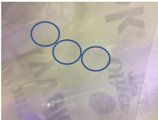
Figure 33 - Example of contamination illuminating under a black light
