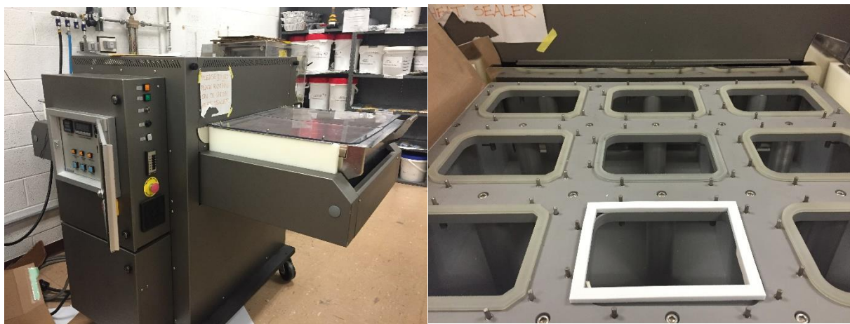
Figure 34 - Shuttle sealer with square seal custom gasket.
