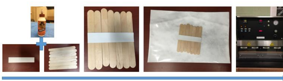
Figure 9 - Filling and sealing process for large pouches
