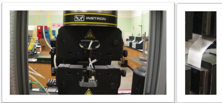
Figure 26 – ASTM F88 Seal strength testing on Instron Universal Test Machine
