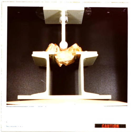
Plate 1. Breaking of Cooked Crosscut Slices Using Breaking Apparatus and Instron Universal Testing Instrument
