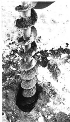
Figure 7. Sample loss from the bottom auger section.
