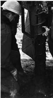
Figure 6. Sampling from the auger tool.
